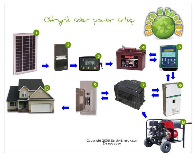
For this system, the generator is meant to undertake the function of the sun. That is, a source of energy whenever it's not available from the sun -- more precisely, during cloudy weather.
