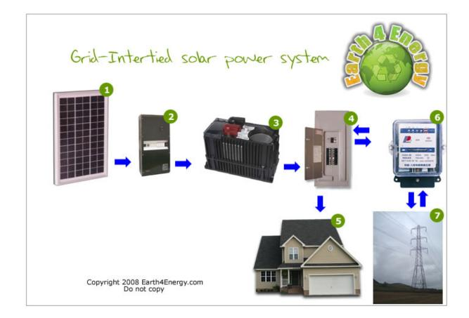
The system is also referred to as an interactive solar electric system, or on-grid system. It is, in fact, a conjoint system, since it entails the partial use of the local power grid. The idea is to observe the proportion of consumed energy versus the one generated by the solar system.
