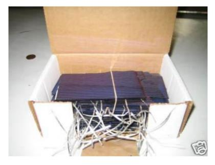
You can also use complete/unbroken cells. In my videos I used full cells produced by Evergreen solar. They put out 1.98 watts per cell. Visit the following link to view all of the new solar cells that are currently available:
