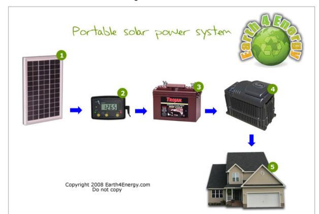
An energy source represented by a solar panel (or several solar panels, as the case may be, that don't need to go beyond 12V), a charge controller, a battery, an inverter, and, finally, an appliance of any kind, are the main elements needed
