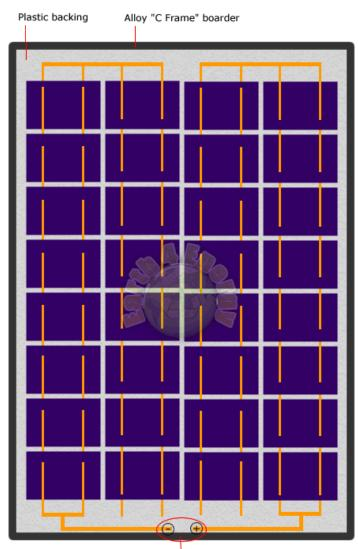
Wires go through backing into a junction box
