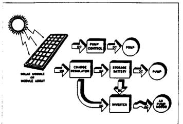
A typical water delivery system may contain one module to hundreds of modules that deliver current to pumping equipment. For continuous pumping, battery storage may be added, but for most applications a battery is not required since solar systems deliver the most water when the sun is brightest.
