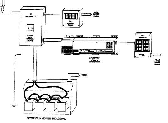
\*This system could easily be configured to 24 volts. However, 12 volt appliances are much easier to locate than 24 volt units. An inverter and common 117 VAC appliances alleviates this problem.
