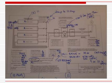
The calculation worksheet (which can be obtained from Brooks Engineering (or other solar PV websites) allows the designer to quickly match the inverter information, the PV panel specifications, temperature & wiring sizes for the entire system. It will help even the plan reviewer note discrepancies or potential problems (recommended, but not required for submittal).
