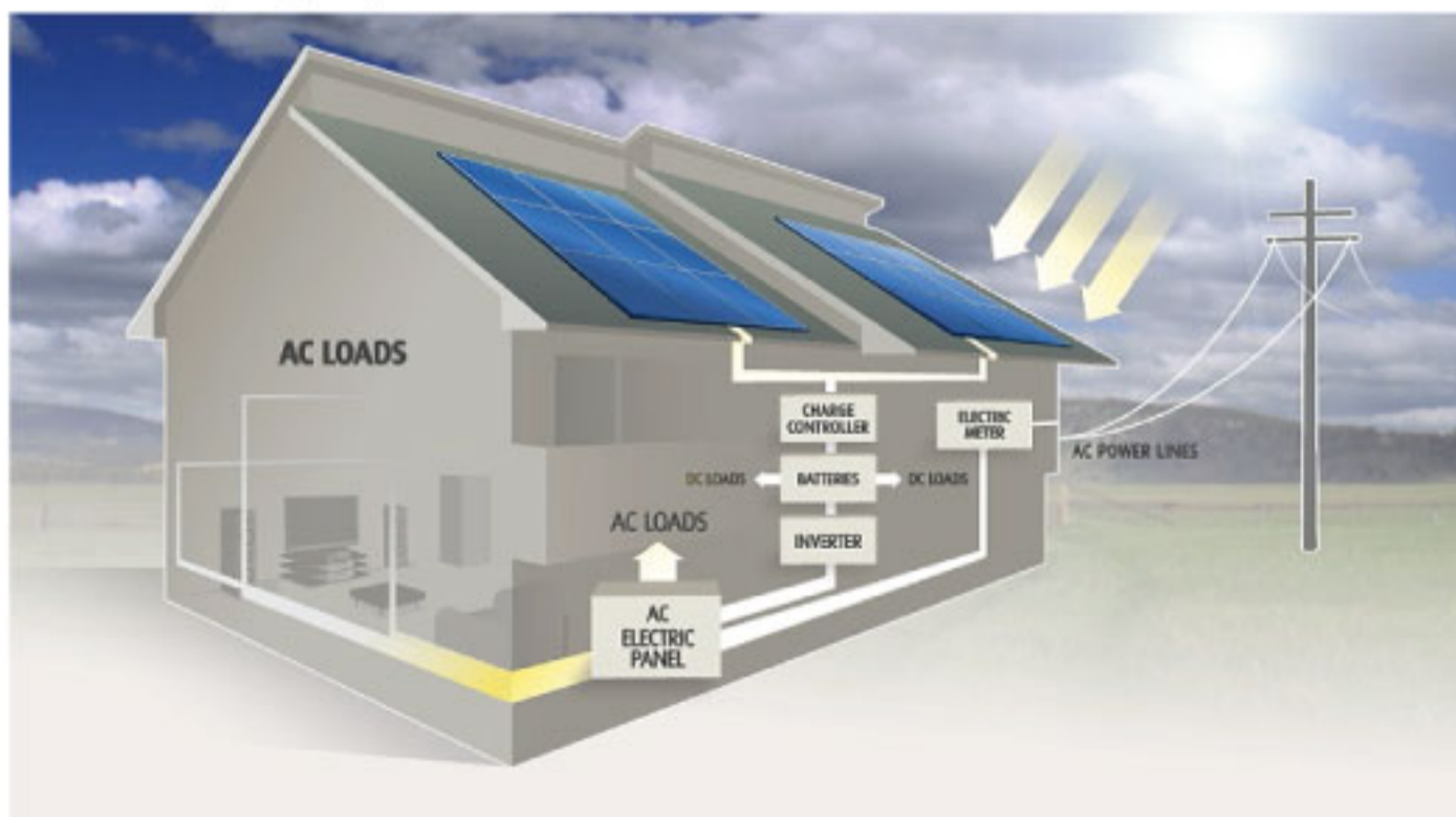
Figure 4 On-grid PV system with a battery bank
