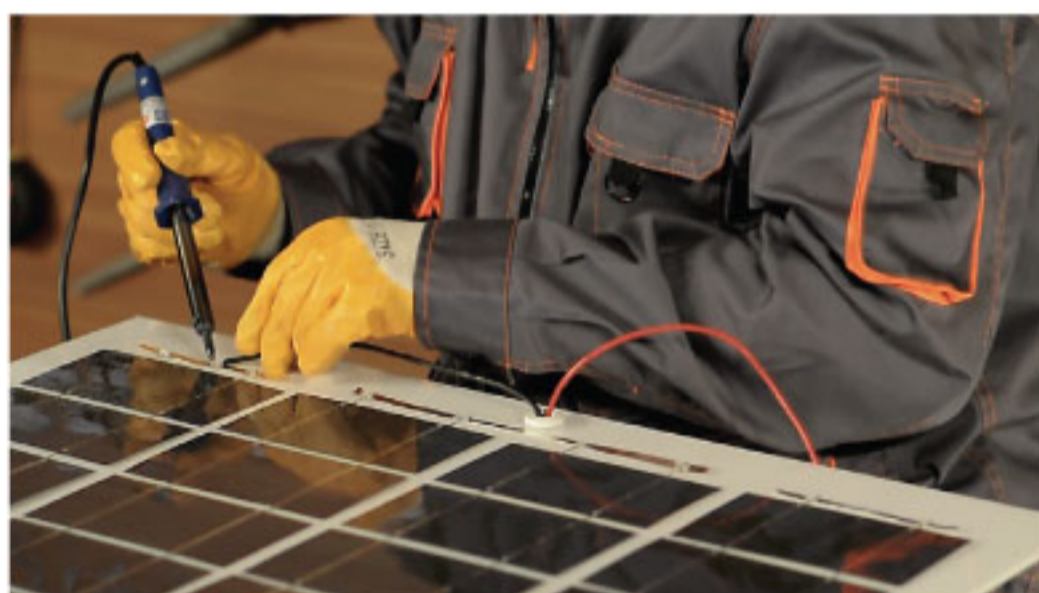
Figure 29 Soldering the unconnected tab wires
