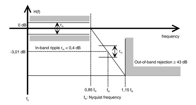
Figure A.1: Half-Nyquist baseband filter amplitude characteristics
