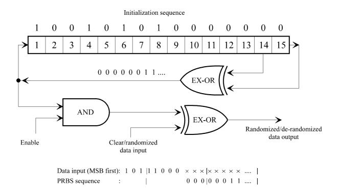
Figure 3: Scrambler/descrambler schematic diagram
