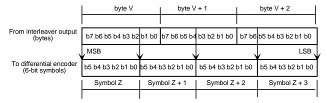
NOTE 1: b0 shall be understood as being the Least Significant Bit (LSB) of each byte or m-tuple.
