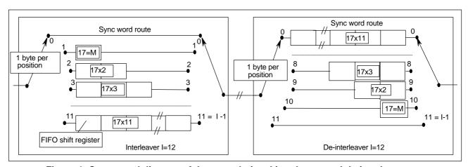
Figure 4: Conceptual diagram of the convolutional interleaver and de-interleaver
