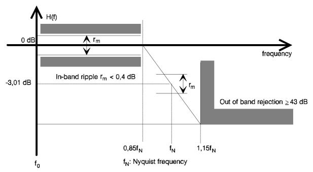
Figure A.1: Half-Nyquist baseband filter amplitude characteristics
