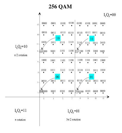
Figure 8: Constellation diagrams for 128-QAM and 256-QAM
