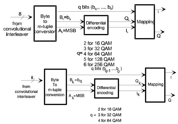
Figure 6: Example implementation of the byte to m-tuple conversion and the differential encoding of the two MSBs
