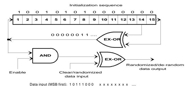
0 0 0 0 0 0 1 1 PRBS sequence Figure 3: Scrambler/descrambler schematic diagram
