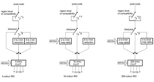
The IRD shall translate a pixel's pseudo-colours into Y, Cr, Cb and T components according to the following model:
