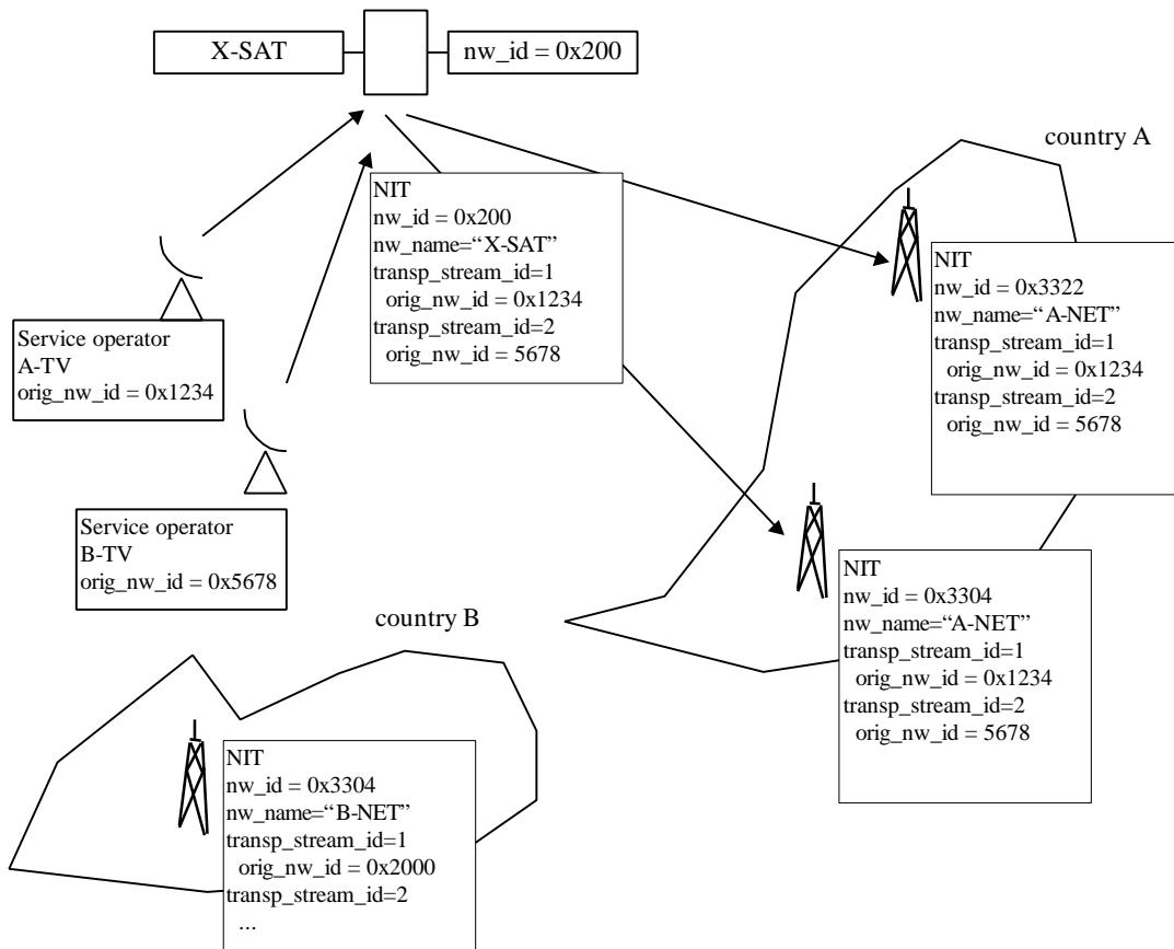
The satellite NIT contains the original\_network\_id of A-TV and the network\_id of X-SAT.
