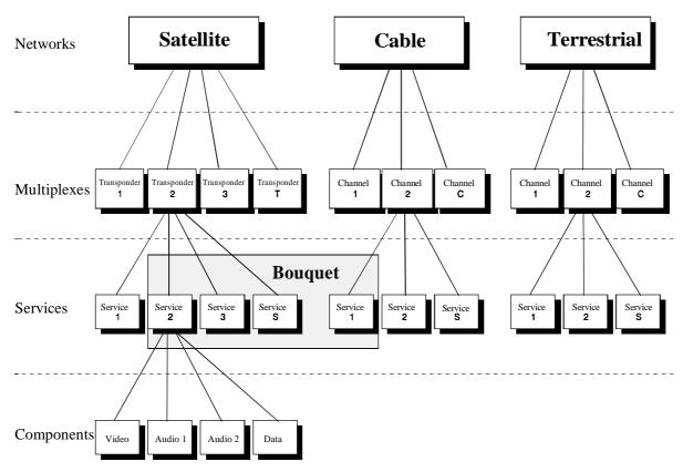
Figure 1: Digital broadcasting, service delivery model
