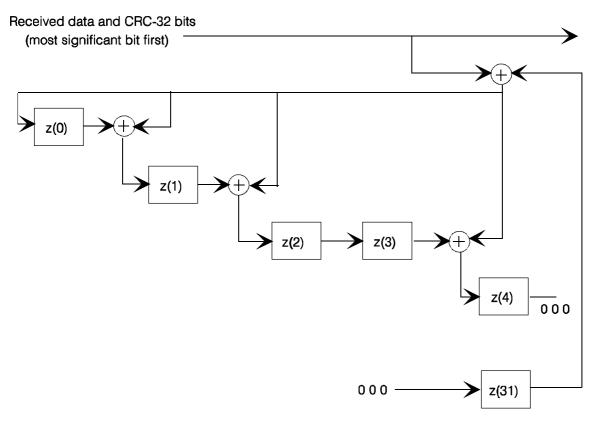
Figure B.1: 32-bit CRC decoder model
