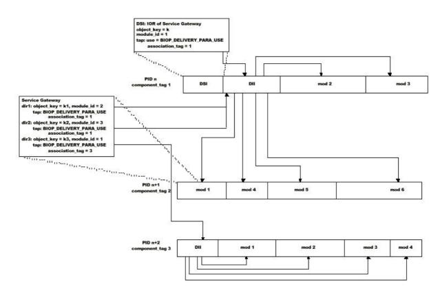
Figure D.1: Object Carousel example
