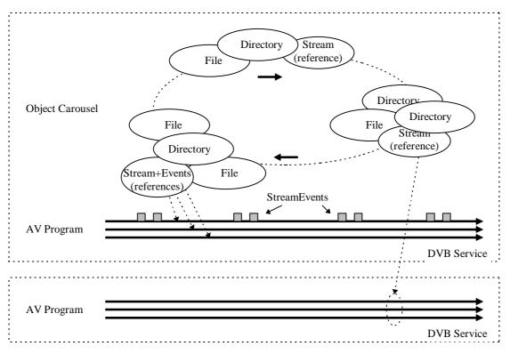
Figure 4.4: Example of including Object Carousel specification in DVB Services
