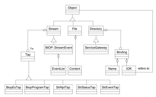
Figure 4.6: Supported Objects within Object Carousel
