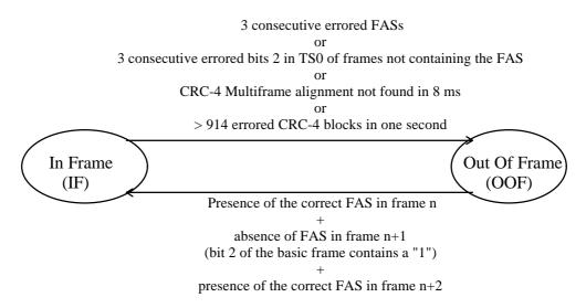
Figure 11: Frame alignment state diagram
