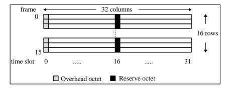
Figure 10: Multiframe at 2 048 kbit/s
