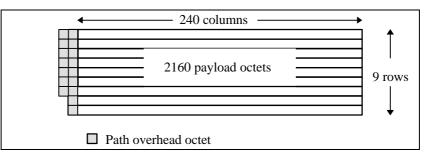
Figure 21: Frame structure at 139 264 kbit/s
