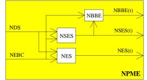
Figure 25: Near-end Performance Monitoring Event (NPME) function
