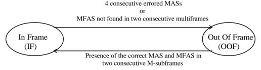
Figure 20: Frame alignment state diagram
