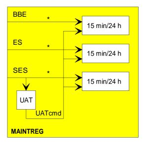
\* The determination of (un)available time introduces (functionally) a delay of 10 seconds. This delay should be considered when counting BBE, ES, SES.
