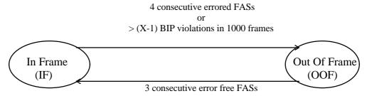
Figure 23: Frame alignment state diagram
