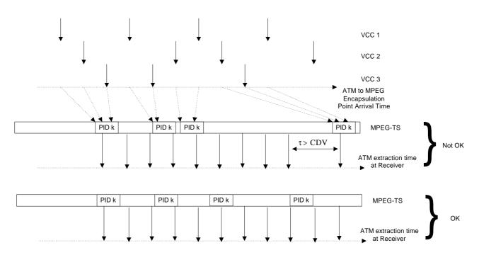
Figure 4: MPEG-TS packets distribution for ATM traffic support
