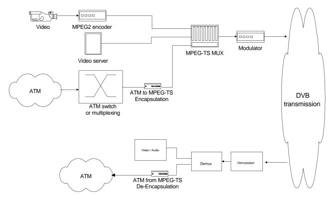
Figure 1: Conceptual DVB/MPEG chain carrying ATM
