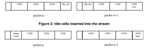
Figure 3: Adaptation fields inserted into the MPEG-TS header
