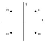
Figure 7: Mapping for the QPSK constellation (downstream OOB)
