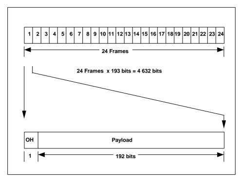
Figure 17: SL-ESF Frame Structure
