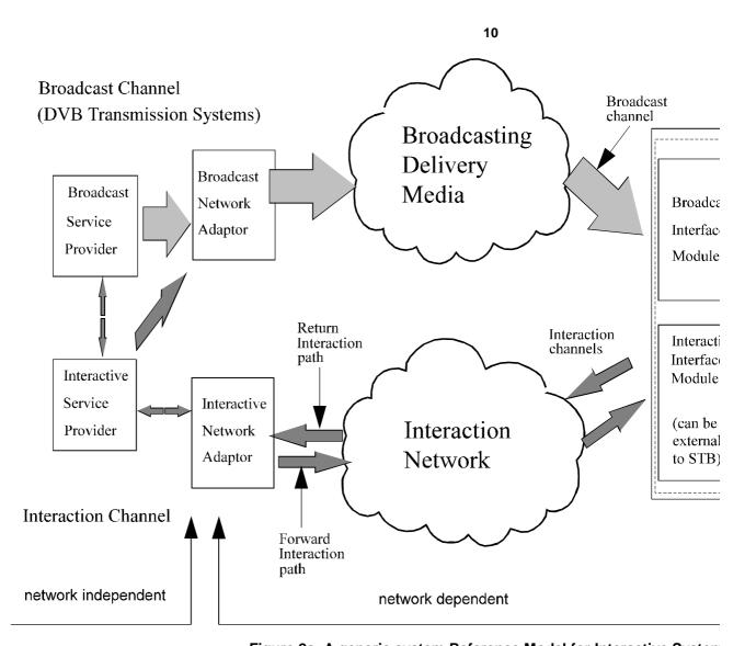
Figure 2a: A generic system Reference Model for Interactive System
