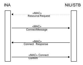
Figure 33: Connection signalling for additional connections
