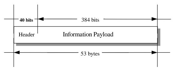
Figure 22: ATM cell format
