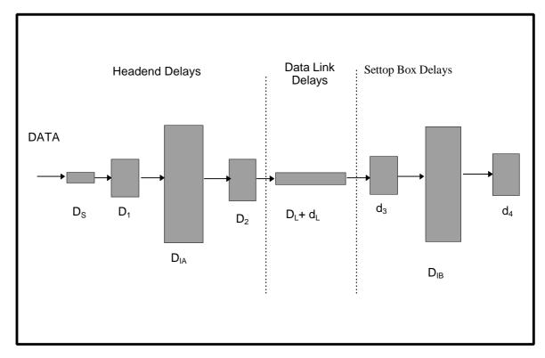
Figure 24: System Model for Timing Analysis
