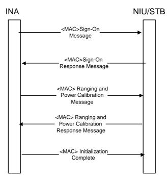
Figure 30: Ranging and Calibration Signalling
