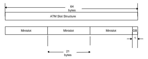
Figure 36: Minislot Framing Structure
