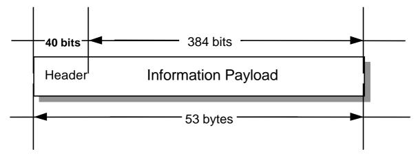
Figure 18: ATM cell format
