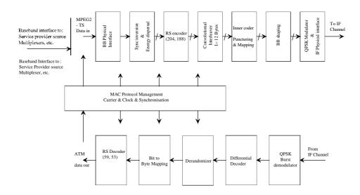
Figure 6: Conceptual Block Diagram for the IB Head-End Transceiver
