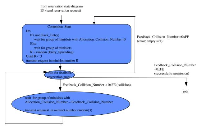
Figure 37: Ternary Splitting Algorithm
