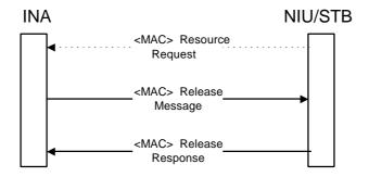
Figure 34: Connection release signalling
