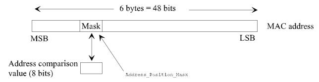
Figure 31: Position of Mask in MAC address
