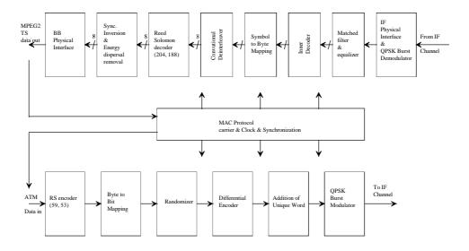
Figure 5: Conceptual Block Diagram for the IB NIU Transceiver
