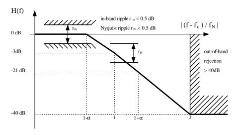
Figure 13: QPSK Upstream Transmitter Power Spectrum
