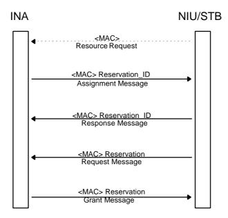
Figure 35: Reservation access signalling
