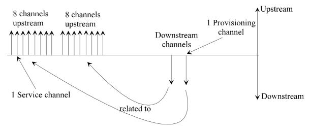
Figure 26: Example of a frequency allocation for the FDM scenario
