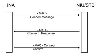
Figure 32: Connection Signalling for the Initial Connection
