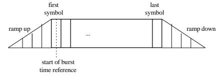
Figure 15: Burst Ramp Up and Down
