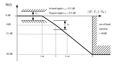
Figure 8: QPSK Downstream Transmitter Power Spectrum
