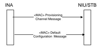
Figure 29: Initialization and Provisioning signalling
