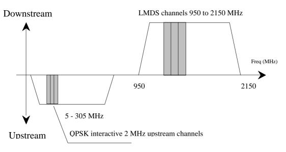
Figure 3b: DVB preferred IF frequency ranges for LMDS interactive systems (IB)
