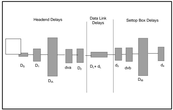
Figure 22. System Model for Timing Analysis
