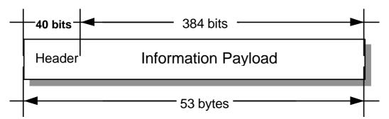
Figure 16: ATM cell format
