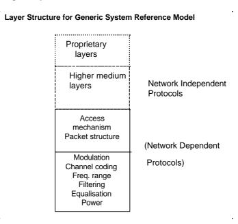
Figure 1: Layer structure for generic system reference model
