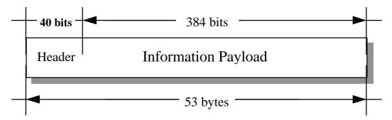
Figure 20: ATM cell format
