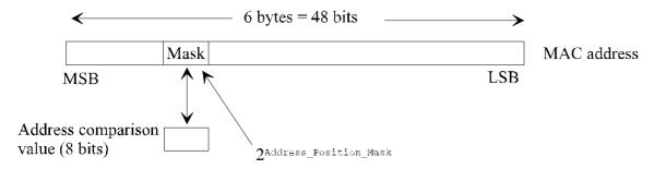
Figure 29: Position of Mask in MAC address
