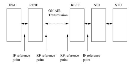
Figure 2 a: position of IF and RF reference points in the particular case of LMDS networks
