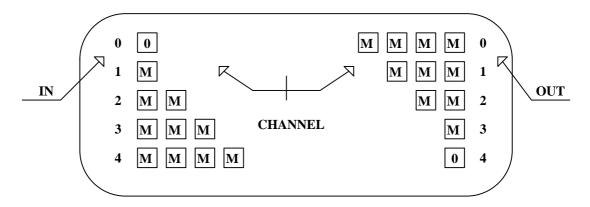
Figure 17: Interleaver and De-interleaver structures
