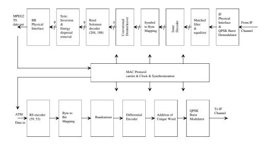
Figure 6: Conceptual Block Diagram for the IB NIU Transceiver
