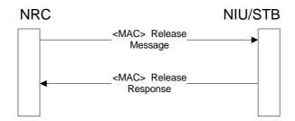
Figure 31: Connection release signalling
