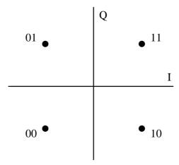
Figure 12: Mapping for the QPSK constellation (upstream)
