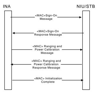
Figure 27: Ranging and Calibration Signalling
