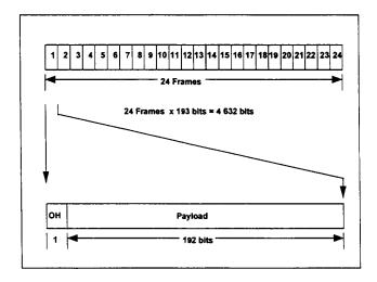
Figure 15: SL-ESF Frame Structure
