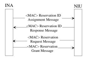
Figure 32: Reservation access signalling
