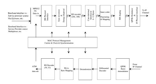
Figure 7: Conceptual Block Diagram for the IB Head-End Transceiver
