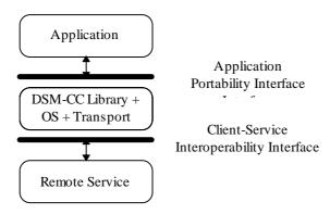
Figure 7: Application and Service Interfaces
