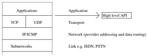
Figure 2: TCP/IP model
