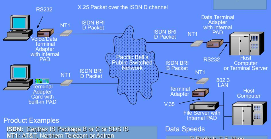
D Packet: 9.6 kbps with up to 15 logical channels
