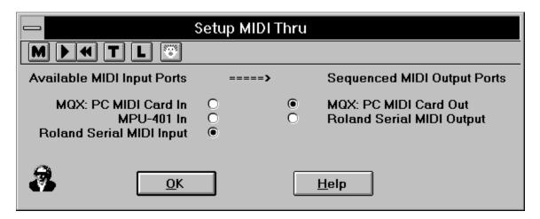
This screen is where you to set up your MIDI Thru options. The top half will eventually allow you to select which MIDI messages to filter—CanvasMan currently filters sysex, system reset, active sensing, and tune request.
