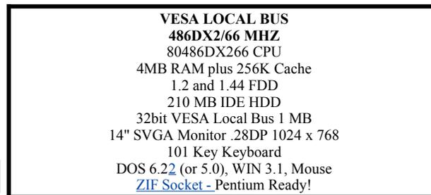
80486DX266 CPU - This computer is based on an Intel 80486DX CPU chip (the heart of the computer) whose speed has been doubled from 33Mhz (it's rated speed) to 66Mhz, but only for internal operations (it won't make your hard drive or video run faster). This is currently "top of the line" reasonable for home systems. There are suddenly lots of players in this Market. TI, CYRIX, AMD, etc. Expect to pay a 10 - 25% premium for Intel.
