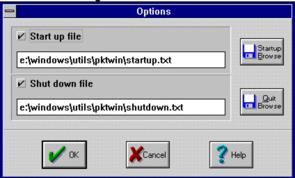
The Initialisation <u>dialogue box</u> controls whether a file is send to the TNC on <u>Start up or Shut down</u> and which files those are.
