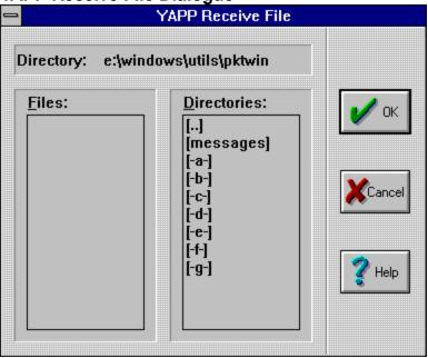
The YAPP Receive File <u>dialogue box</u> is for selecting a directory in which to store the file to be down loaded. The file name for the file will be supplied by the station sending the file.
