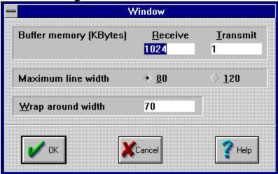
The Window dialogue box allows you to control how the <u>Transmit</u> and <u>Receive</u> windows are set.
