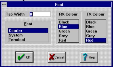
The Font <u>dialogue box</u> controls which font, which colours and the Tab settings for the text used by the program.
