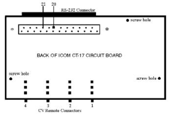
Take one of the mini-plug cables that comes with the ICOM CT-17 and cut one end off. Either run the wire through one of the unused CV Remote Connectors (1,2,3, or 4) or through a hole you drill in the case. Strip the two exposed wires and solder to pins 20 and 22 shown above. The other end of the cable plugs into the R-7100 Recorder Remote Jack.
