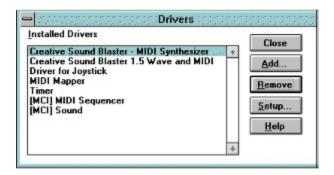
The third line shows the Driver for Joystick provided with this program and is installed as an "Unlisted or Updated Driver" after pressing the Add.. button.
