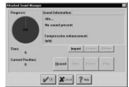
Figure 4-9. The Attached Sound Manager dialog box features controls for recording, importing, and playing sound clips in a media library.
