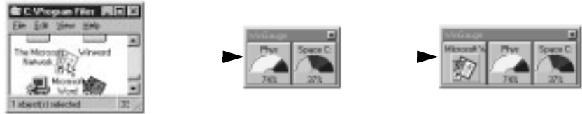
Figure 3-1. Drag an application icon into the WinGauge window to add it as an Action gauge; click an Action gauge to launch the application
