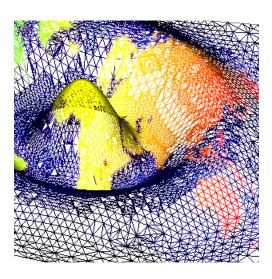
The wire frame or Adaptive Mesh Technology from AIST fits the requirements exactly. Where minor deformations have taken place the wire frame is regular. The wire frame becomes more complex and structured if deformations are more complex.
