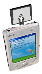
3 When your handheld emts a two-tone beep you have properly removed the card. Reinsert the dummy CF card to protect the connectors.
