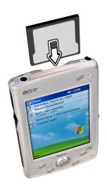
4 Push the card into the slot using your finger until you feel the card lock and hear an audible system sound; this will signal that the card is already properly seated within the slot.
