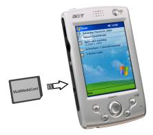
3 Push the card into the slot using your finger until you feel the card lock and hear an audible system sound. This indicates that the card is properly seated within the slot.
