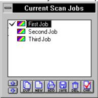
A scan job is simply a task that you designate the scanner to process and scan. For instance, when you first preview an image, the image as a whole has its own parameters (its own brightness and contrast setting, resolution, etc.). The whole image can be treated as one scan job, or you can select a part of the image, apply different parameters to it, and treat that as a separate scan job. Scan Job 1 can be in color mode, while scan job 2 can be in grayscale mode.
