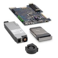
AppleCare Service Parts Kits for Xserve include a power supply, blower, logic board, and Apple Drive Module.
