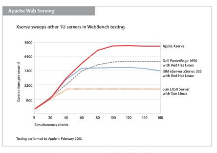
Xserve running Apache on Mac OS X Server outperforms all three other 1U servers running Apache on Linux operating systems. Xserve is 29 percent faster than the Dell PowerEdge 1650, 47 percent faster than the IBM eServer xSeries 335, and nearly three times as fast as the Sun LX50 Server. These results demonstrate the benefit of the high-throughput Xserve architecture, optimized for demanding server tasks.
