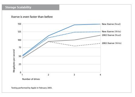
A scalable storage architecture, with four independent ATA/133 drive channels, allows Xserve storage throughput to increase as you add more drives. On Xserve with a single drive, Bonnie reports a read speed of 52MB/s, versus the 46MB/s on the original Xserve. As the number of drives increases, the performance of Xserve improves linearly up to a peak of 150MB/s—a throughput that's 30 percent higher than the original Xserve.
