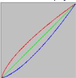
This panel shows the tonal reproduction curve of the red, green, and blue colors of your display. This panel reflects any change you make with the **Color temperature** and **Contrast** sliders.
