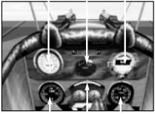
RPM SLIP INDICATOR SPEED
