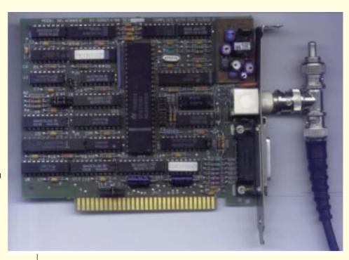
Network card with terminator, cable and "T" piece
