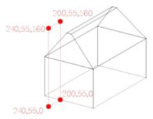
The first roof surface of the tower can be entered with absolute coordinates.
