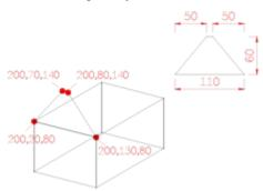
You could draw the inclined gable by entering all the coordinates however all the corner points can be snapped onto with the object snap options.
