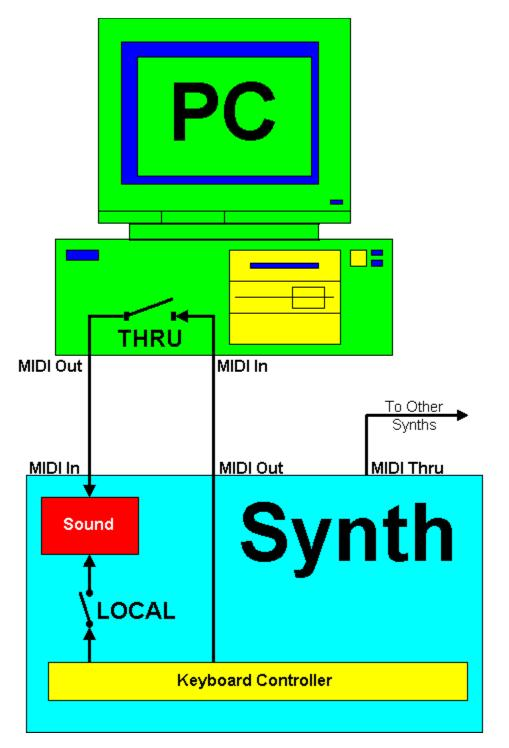
Study the diagram—it shows the 'correct' way to connect your MIDI cables. Once you have connected things this way, you should turn **PowerJam Central**'s Thru On and Local Off. (If you're running **PowerJam Central** at the same time as your sequencer, however, leave **PowerJam Central**'s Thru Off and turn your sequencer's Thru On.)
