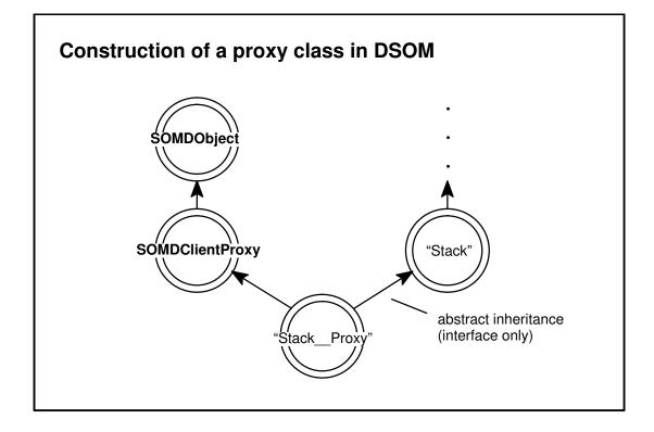
In the newly derived proxy class, DSOM overrides each method inherited from the target class with a "remote dispatch" method that forwards an invocation request to the remote object. Consequently, the proxy object provides location transparency, and the client code invokes operations (methods) on the remote object using the same language bindings as if it were a local target object.
