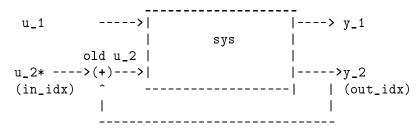
The input that has the summing junction added to it has an \* added to the end of the input name.
