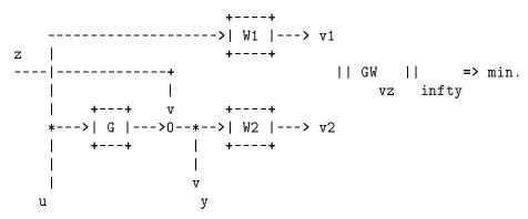
The closed loop system GW from [z; u]' to [v1; v2; y]' can be obtained by (all SISO systems):
