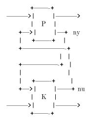
If ny and nu "consume" all inputs and outputs of K then the result is a lower fractional transformation. If ny and nu "consume" all inputs and outputs of P then the result is an upper fractional transformation.
