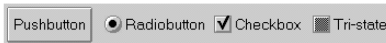
Figure 7.1: This figure shows (from left to right) the following Buttons types: Pushbutton , Radiobutton , Checkbox and Tri-state Button .
