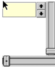
Figure 2.9: This figure shows a horizontal and a vertical slider and a spinbutton
