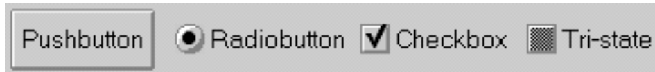
Figure 2.1: This figure shows (from left to right) the following Buttons types: Pushbutton , Radiobutton , Checkbox and Tri-state Button .
