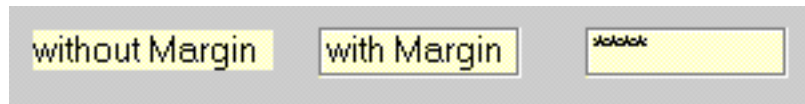
Figure 2.5: In this figure you can see (from left to right) an EntryField without a margin, one with a margin and an EntryField with margin and the style option BS_UNREADABLE
