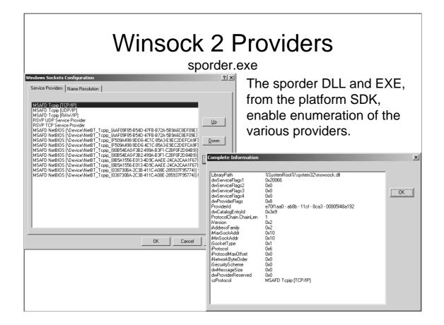
The above is a screen shot of the "SPOrder.EXE", provided as part of the platform SDK. This small utility displays the service providers registered under winsock. Note both classes – "Service Providers" (i.e. Transport Service Providers) and "Name Resolution" (Namespace Service Providers).
