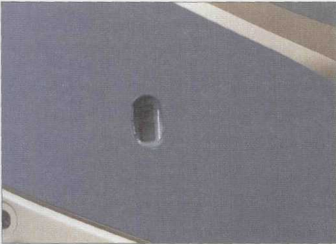
5 On some models, the rear reservoir is visible through an inspection hole in the fairing.
