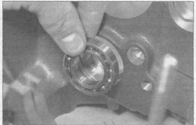
34.10 ... and remove the bearing
