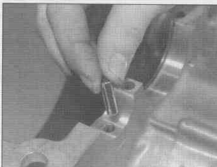
32.5a There's a dowel at one end of each shaft - be sure it's installed in the case ...
