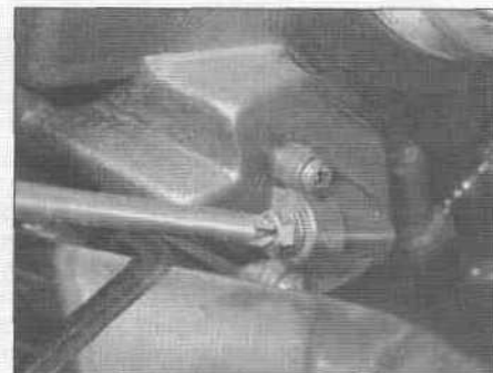
8.4 Turn the vertical adjuster to move the beam up or down
