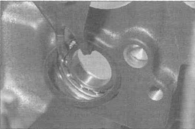
34.9 Remove the bearing snap-ring from the case ...
