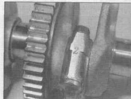
30.2 This number mark indicates the connecting rod bearing size - you'll need to make your own marks indicating cylinder number
