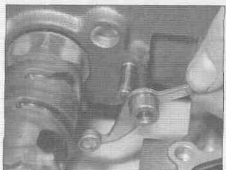
34.5b ... and slide the shift cam stopper off the bolt
