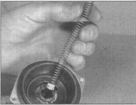
8.52 Lift out the diaphragm spring and spring seat
