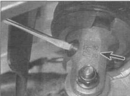
15.18 Turn the adjuster and count the clicks to set rebound damping force; standard settings for rebound (R) and compression (C) are stamped in the shock (arrowed)
