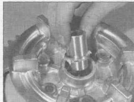
15.7 Remove the spacer from the other side of the coupling
