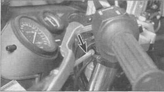
14.6 Loosen the upper pinch bolts on each fork (arrow)
