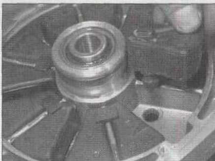
Cush drive rubbers dampen out transmission shocks
