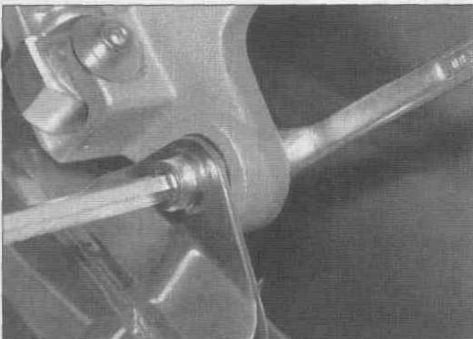
13.4 Remove the muffer mounting bolts at the rear foot pegs
