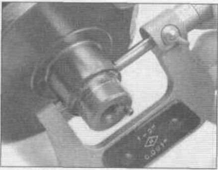
29.13 Measure the diameter of each crankshaft journal at several points to detect taper and out-of-round conditions
