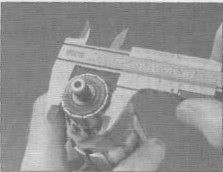
24.10 Check the commutator for cracks, discoloring and wear
