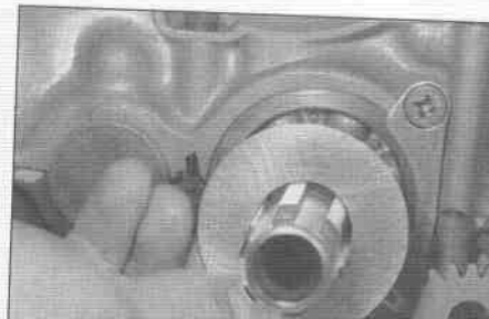
19.12u ... the alternator and oil pump drive gears ...
