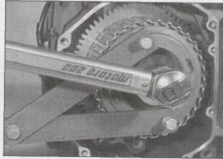
19.12f Hold the pressure plate from turning with a special tool (see Tool Tip) and loosen the diaphragm spring holder nut with a 50 mm socket...
