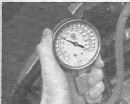
6.5 A compression gauge with a threaded fitting for the spark plug hole is preferred over the type that requires hand pressure to maintain the seal
