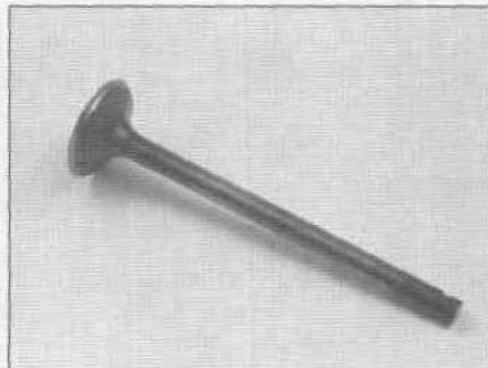
13.17 Check the valve face, stem and keeper groove for signs of wear and damage
