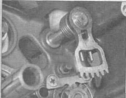
24.8 ... then pull the gearshift shaft out of the engine
