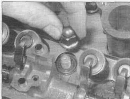
11.8c Lift off the cylinder head nuts - some of the studs have cap nuts, like the one shown here ...
