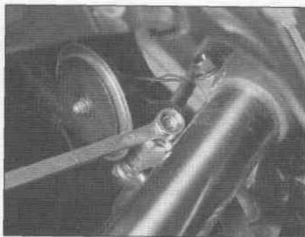
9.3b ... and this type is used on Katana 600/GSX600F and Katana 750/GSX750F models - use a six-point box wrench (ring spanner) on the banjo bolts and be prepared for some leakage
