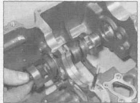
34.8 Slide the shift cam out of the case
