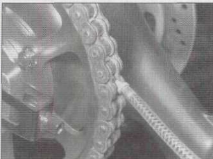
1.4 Apply 20W/50 engine oil to the joints between the side plates and the rollers - not in the center of the rollers
