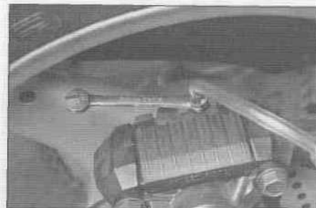
10.6a ... and place a box wrench (ring spanner) and vinyl tube on the valve (Katana/GSX-F rear caliper shown; GSX-R rear caliper similar)...
