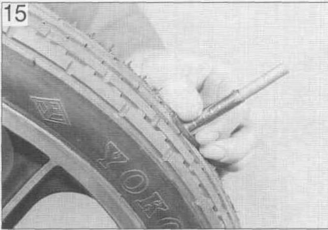
Checking the tyre tread depth
