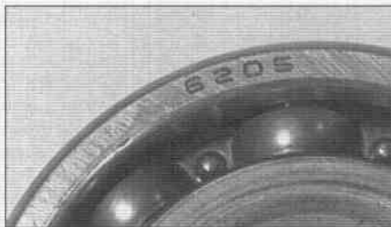
5.16 Typical bearing marking
