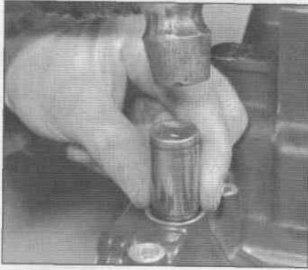
24.14c ... and tap the seal in with a socket the same diameter as the seal
