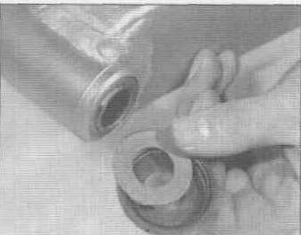
14.3 Pry the seals out with a screwdriver and remove the washer behind each seal
