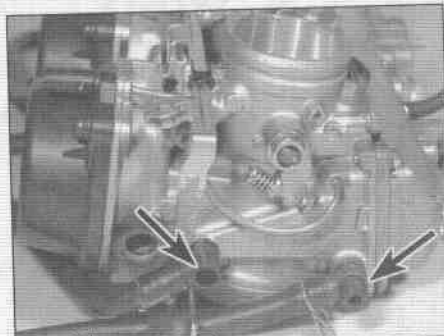
8.49 Pull the carburetors out of the fuel and vent lines (arrowed) to separate them
