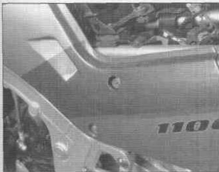
2.1 The seat lock is operated by the ignition key
