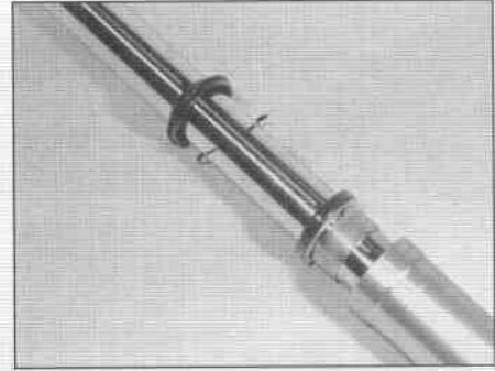
8.73 Separate the inner and outer fork tubes to expose the oil seal and guide bushing
