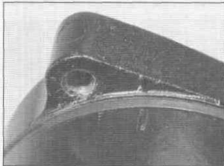
24.2 Check for alignment marks where each end cover meets the starter - make your own marks if the factory marks aren't visible
