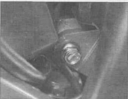
11.4 Remove the nut from the shock absorber upper bolt...
