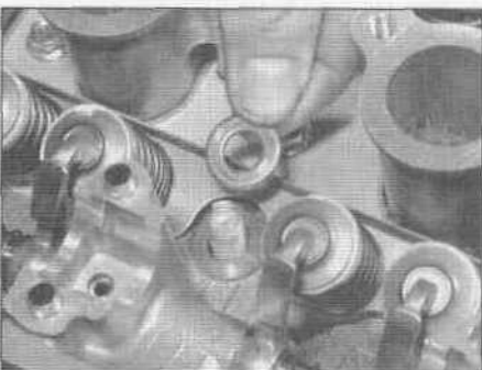
11.8d ... some of the nuts have copper washers, some have steel washers and some have no washers (depending on model); label the nuts and washers so they can be reinstalled on the correct studs
