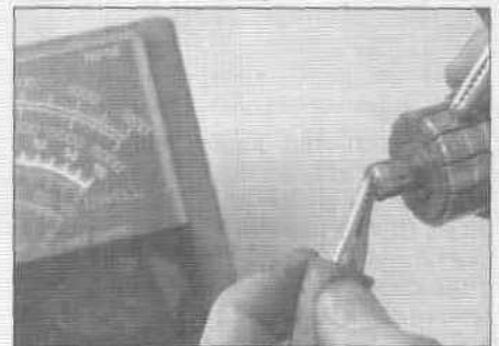
24.11b There should be no continuity between the commutator bars and the armature shaft
