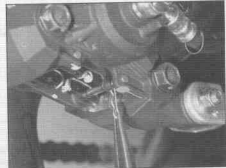
3.3 Pull the clips out of the pad retaining pins
