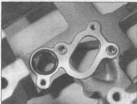
18.7a Make sure the pump dowels are in their holes; remove the small O-ring ...
