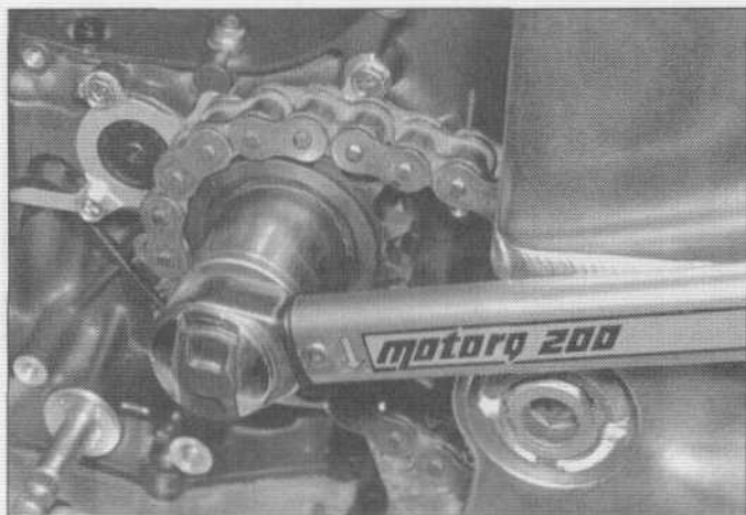
17.9d ... tighten the nut to the correct torque ...
