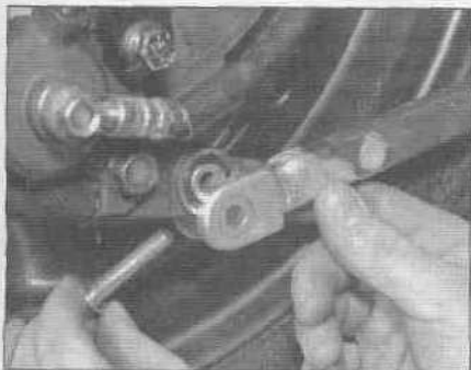
4.2c ... and withdraw the bolt to separate the torque rod from the caliper (this is a GSX-R caliper)
