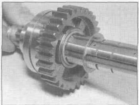
33.4n ... slide off the thrust washer ...
