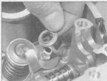
13.23a On all models, install the lower spring seat on all valves (be sure not to confuse the spring seat with the spring retainer, which goes on top of the spring)
