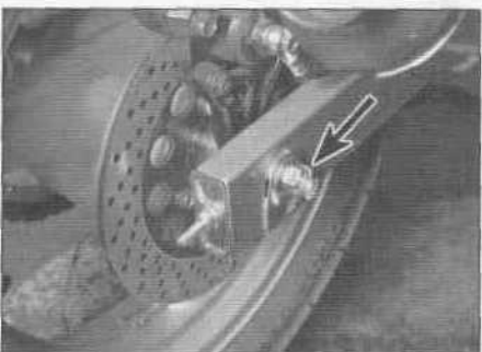
14.5a If the axle nut is equipped with a cotter pin (arrowed), remove it - use a new cotter pin during installation
