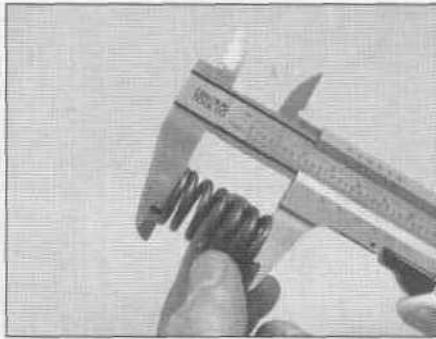
19.14 Measure the clutch spring free length (coil spring clutch)
