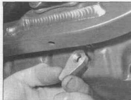
5.26 This type of nut has a tab that prevents it from turning when the bolt is tightened
