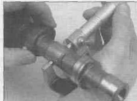
10.16b Measure the cam bearing journal with a micrometer
