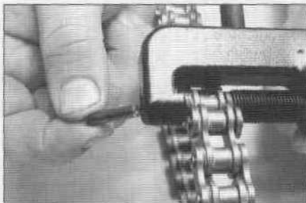
8.2 ... withdraw the pin, remove the tool...
