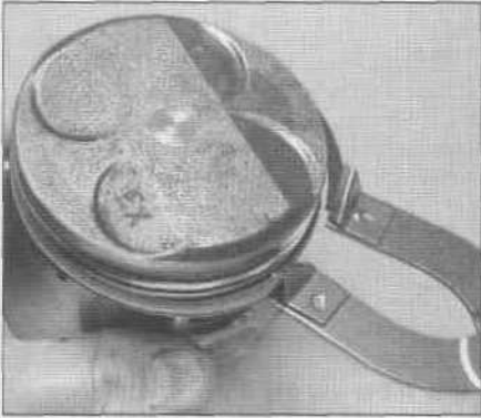
15.6 Remove the piston rings with a ring removal and installation tool
