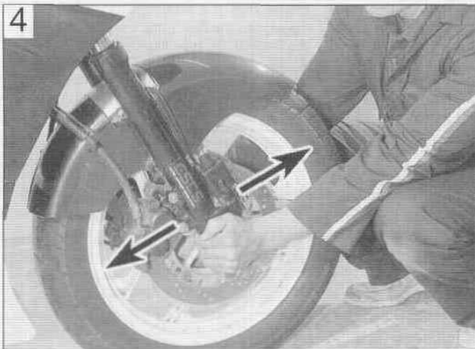
Checking the steering head bearings for freeplay
