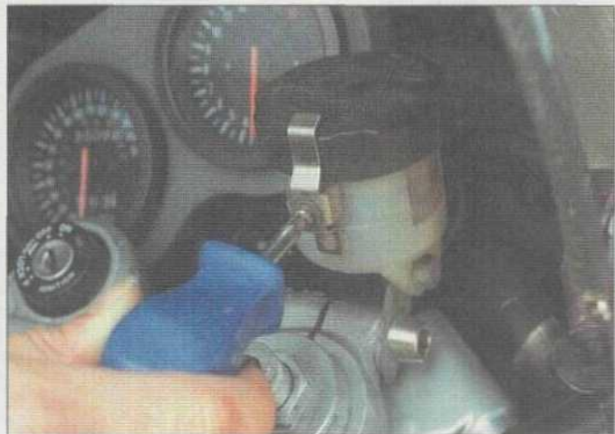
2 On models with a screw top cap (on other models the cap will be held by two screws), remove the security clamp . . .
