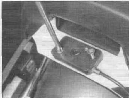
2.4 ... and the latch screws, then undo any tie wraps that secure the lock cable
