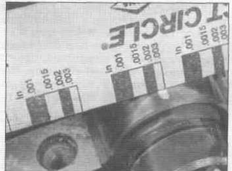
29.11 Measuring the width of the crushed Plastigage (be sure to use the correct scale - standard and metric are included)
