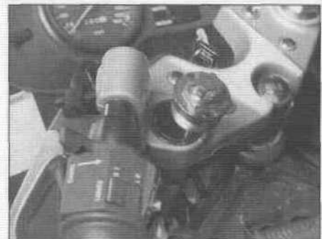
16.2 Lift out the fork cap bolt and inspect its O-ring
