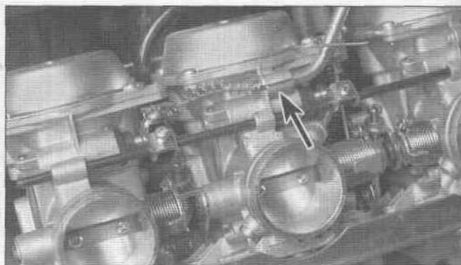
11.2 Separate the choke cable housing from the bracket at the carburetor (arrowed)
