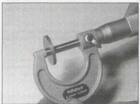
Tappet shims are measured with a micrometer
