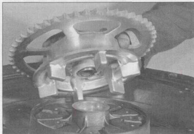
18.2 Lift the sprocket and hub from the rear wheel
