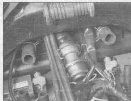
14.16 The air switching valve is mounted beneath the air suction valves
