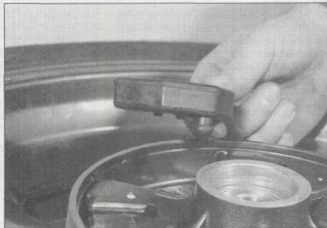
18.3 Pull the damper segments out of the recesses
