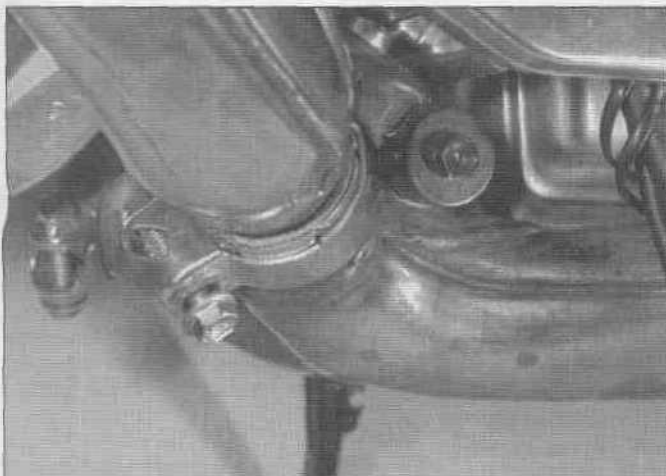
13.2 Loosen the muffer clamps if you plan to separate the mufflers from the pipes
