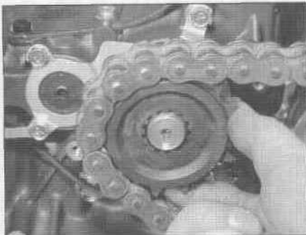
17.9a Engage the chain with the sprocket and slip the sprocket onto the shaft...
