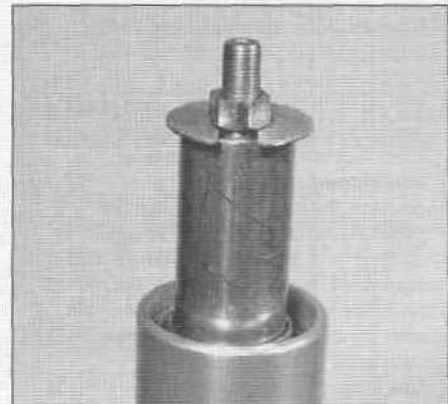
8.69a After you've unscrewed the fork cap, loosen the locknut, then remove the special tool or washer ...
