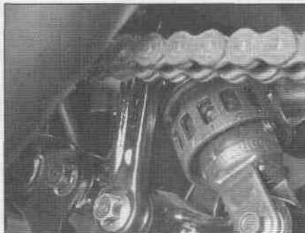
15.25a Turn the adjuster ring on the shock absorber to set spring preload
