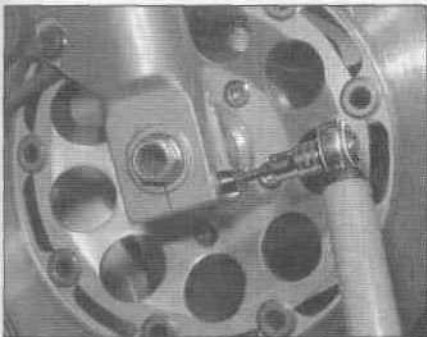
13.11 Loosen the fork pinch bolts ...
