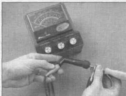
2.5 Unscrew the spark plug caps from the plug wires and measure their resistance with an ohmmeter
