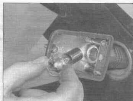
9.2d On all models, press the bulb into the socket and turn it counterclockwise (anticlockwise) to remove
