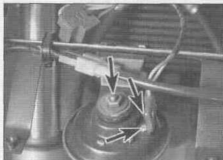
21.1 Disconnect the wires and remove the mounting nut (arrowed) to detach the horn from the bracket
