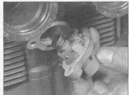
9.4 Install the tensioner body in the engine with a new gasket
