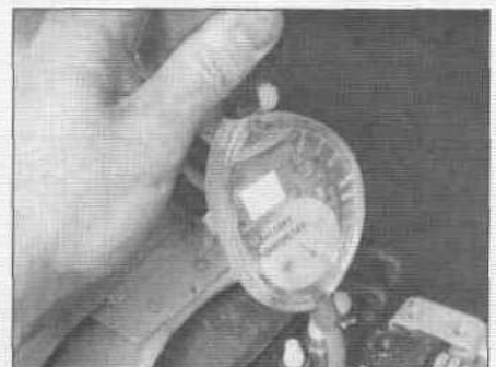
19.7 Check the specific gravity with a hydrometer
