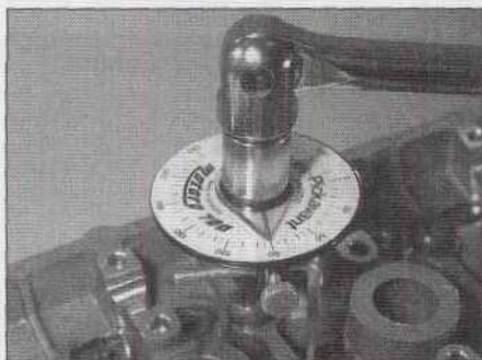
Angle-tightening cylinder head bolts
