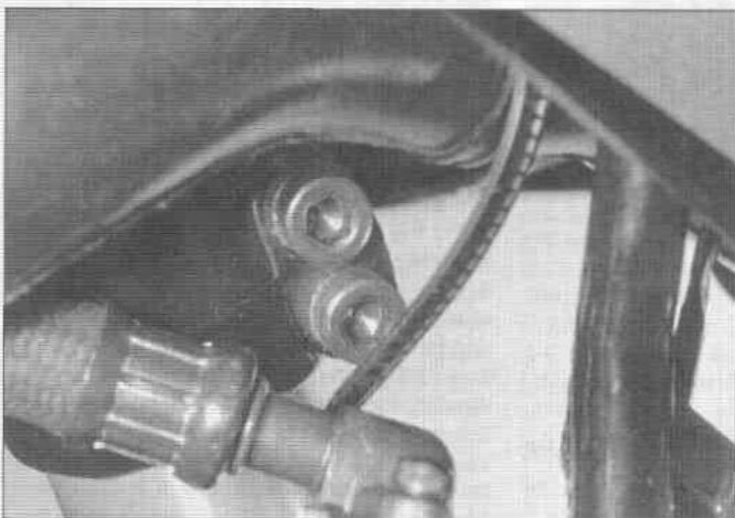
6.9b ... and the lower triple clamp bolts (late GSX-R1100 shown)...
