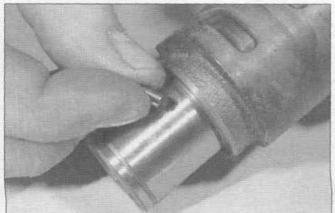
34.11b ... and remove the stopper plate pin from the shift cam
