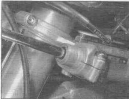
10.3c The damper is secured to the fork tube by a clamp
