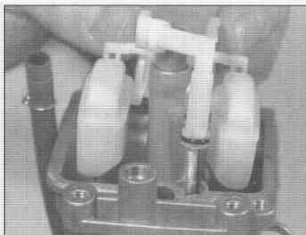
9.7 When installing the floats on BST33SS, BST36SS, BST38SS or BST40SS carburetors, slide the tube and O-ring into the body passage
