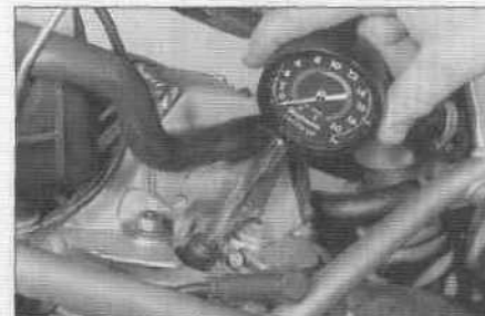
3.20 Using a rubber-cone type cylinder compression gauge
