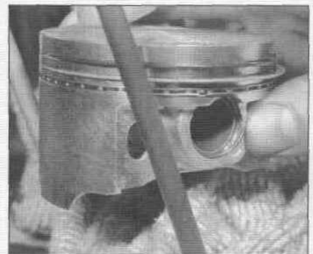
15.17 Install the circlip and make sure it's securely seated in the groove
