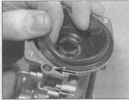
8.53 Carefully separate the diaphragm from the carburetor body and lift it out; also remove the O-ring (arrowed)
