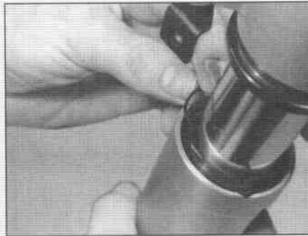
8.72b ... and slip the retaining ring up the fork tube
