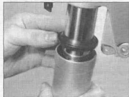
8.71 Pry the dust seal out of its bore with a small screwdriver (be careful not to scratch the fork tube)
