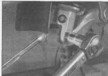
11.5 ... and from the lower bolt, then support the swingarm and remove the bolts
