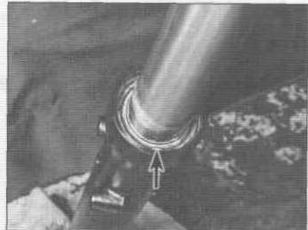
7.8a Pry the retaining ring (arrowed) out of its groove ...
