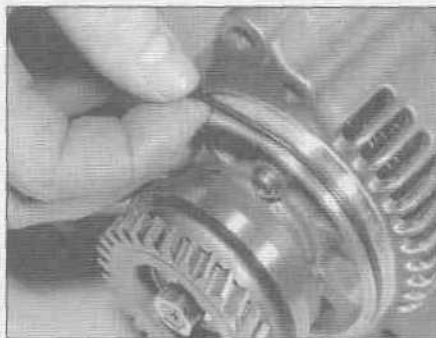
27.8 Remove the O-ring - use a new one during installation
