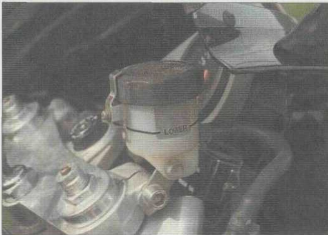
1 Look closely at the inspection window in the master cylinder reservoir. Make sure that the fluid level is above the Lower line on the reservoir.
