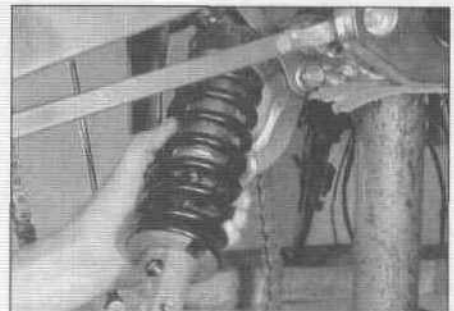
11.7 Lift the shock absorber out of the frame; guide the remote reservoir (if equipped) out at the same time
