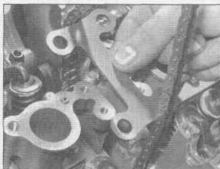
11.9 On late GSX-R 1100 models, lift off the cylinder head plate after the nuts have been removed
