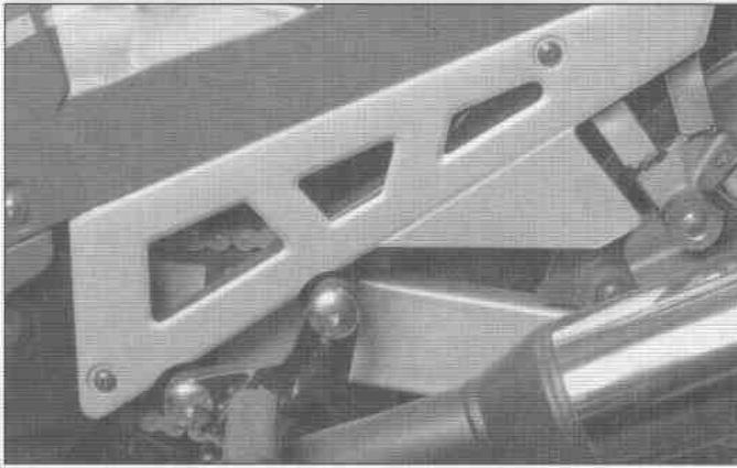
6.2a The side covers are secured by Phillips screws . . .
