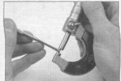
3.10 ... then measure the gauge with a micrometer
