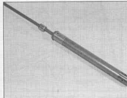
8.77 Check the cartridge for wear or damage; don't try to disassemble it
