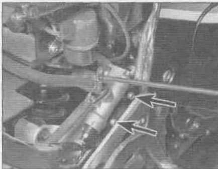
8.3 Disconnect the master cylinder fluid line and immediately direct it into a container to catch the fluid - diagonally mounted master cylinders are secured to the frame by two bolts (arrowed)
