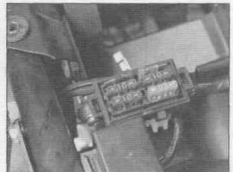
5.1c Unclip the cover to expose the fuses...
