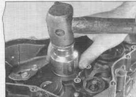
5.2 Using a large socket against the bearing's outer race
