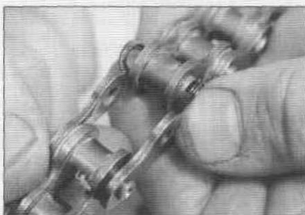
8.3 ... and separate the chain link
