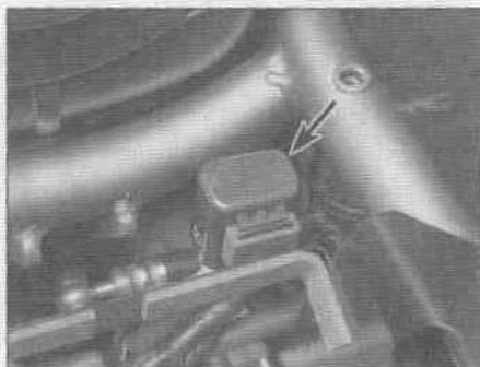
10.3a The turn signal flasher (arrowed) is mounted under the seat - this is a Katana 1100/GSX1100F flasher
