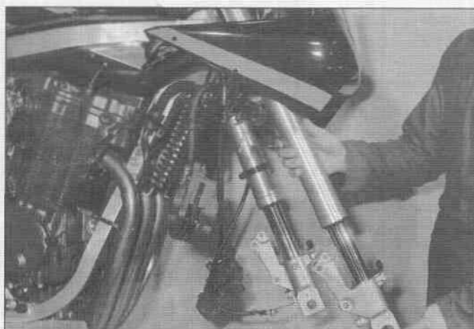
6.9c ... and lower the fork away from the machine
