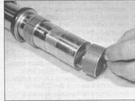
8.74b Slide the bushing off; install a new one during assembly
