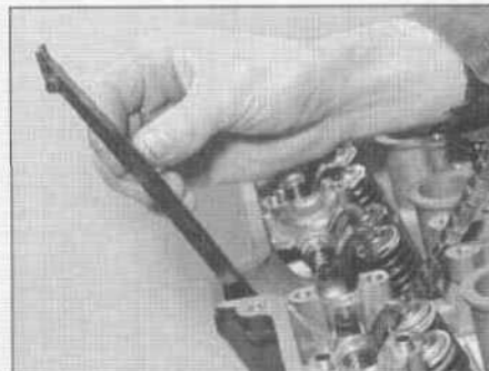
10.9 Lift the chain guide out
