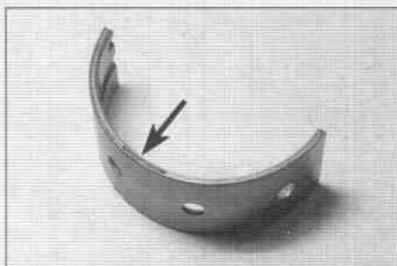
5.14 Shell bearings are either plain or grooved. They are usually identified by colour code (arrow)
