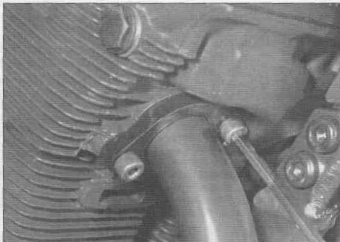
13.5 Unbolt the exhaust pipes from the cylinder head
