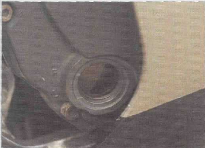
1 With the engine off and the motorcycle upright, check the oil level in the window located at the lower part of the right crankcase cover. The oil level should be between the F (full) and L (low) level marks next to the window.
