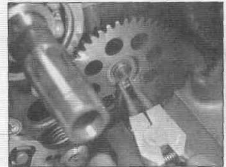
26.7a Remove the oil pump drive gear snap ring ...
