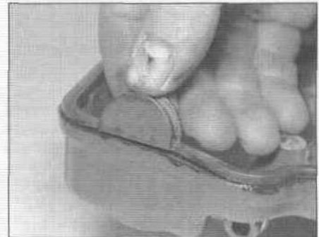
8.11 Be sure the gasket seats securely in the groove
