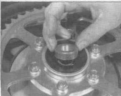
15.6 Lift off the spacer and pry out the grease seal
