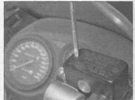
6.3 If you're going to remove the master cylinder cover, loosen the cover screws (it's easier to do this when the master cylinder is still bolted to the handlebar)
