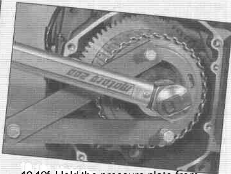
19.12f Hold the pressure plate from turning with a special tool (see Tool Tip) and loosen the diaphragm spring holder nut with a 50 mm socket...
