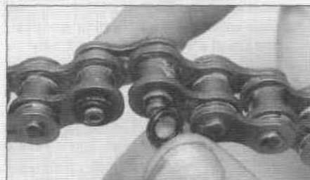
8.5 ... install the O-rings over the pin ends ...
