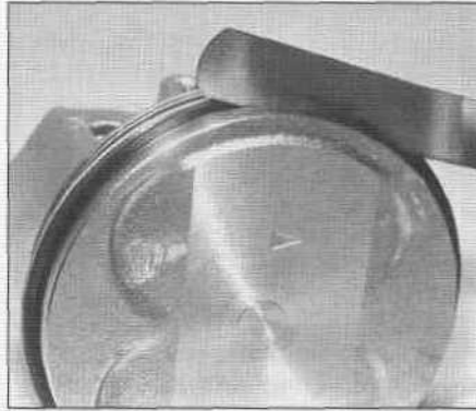
15.13 Measure the piston ring-to-groove clearance with a feeler gauge
