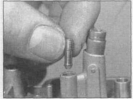
8.64 Unscrew the pilot jet
