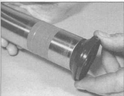
8.53a Wrap the guide bushing on the inner fork tube with vinyl tape so the bushing won't scratch the seal lips during installation (don't forget to remove the tape after the seals are installed)
