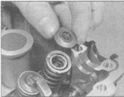
Install the spring retainer, then compress the springs and install the keepers...
