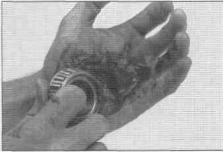
9.23 Work the grease completely into the rollers
