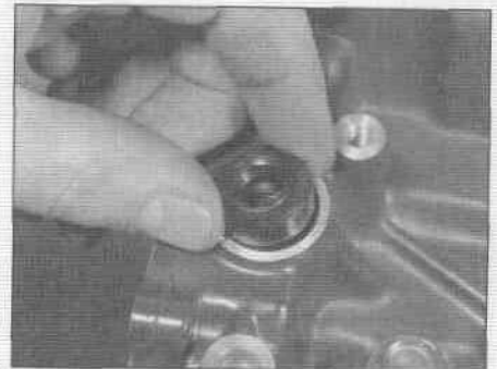
24.14b ... position a new one in the bore with its lip facing into the engine ...
