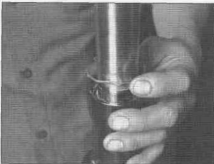
7.8b ... and slide it off the inner fork tube
