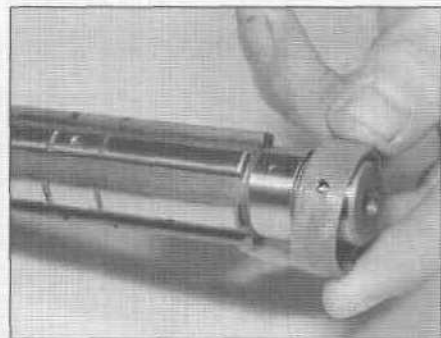
33.10b Align the oil hole of the second driven gear bushing with the oil hole in the shaft
