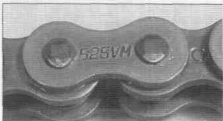
8.10 Typical chain size and type marking
