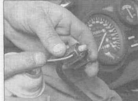
13.3a Lubricating a cable with a pressure lube adapter (make sure the tool seats around the inner cable)
