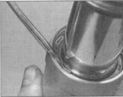
8.72a Pry one end of the retaining ring out of its slot...
