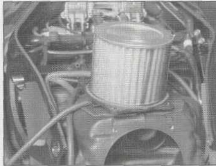
2.17b ... and lift the filter element out of the airbox
