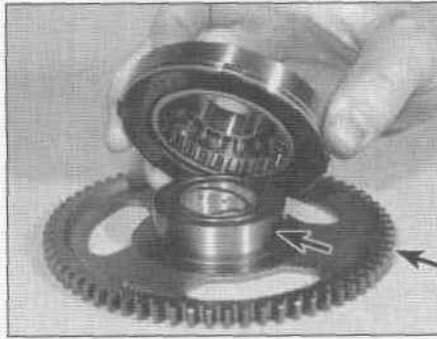
25.11 Inspect the friction surface and the driven gear teeth (arrows)
