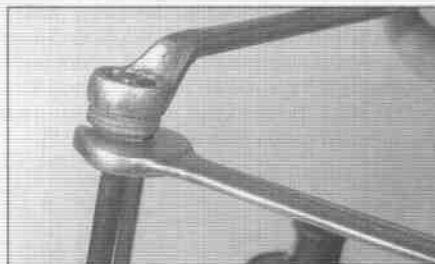
2.18 Two nuts can be locked together to unscrew a stud from a component
