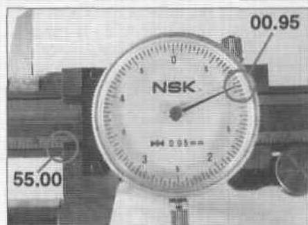
3.14 Vernier gauge reading of 55.95 mm
