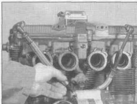
7.3 Remove two bolts that secure each oil hose fitting to the valve cover
