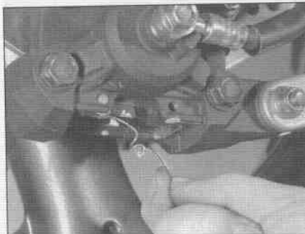
3.5a Pull the anti-rattle spring out of the remaining pin ...
