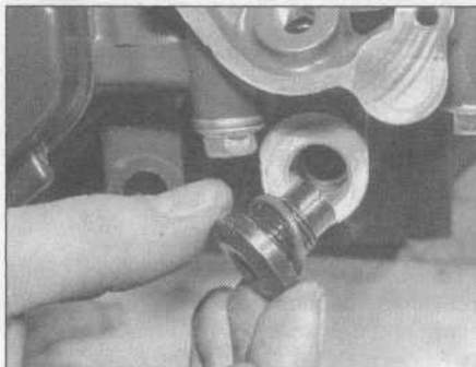
26.10 Remove the main oil gallery plug and O-ring (use a new O-ring during installation)
