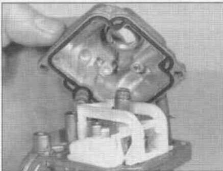
8.59 Remove the float chamber body screws (they're secured with thread locking agent, so you'll need an impact driver and may have to replace them), then lift off the float chamber body and O-ring
