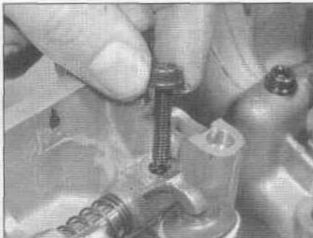
10.34 Remove the rocker shaft lockbolts
