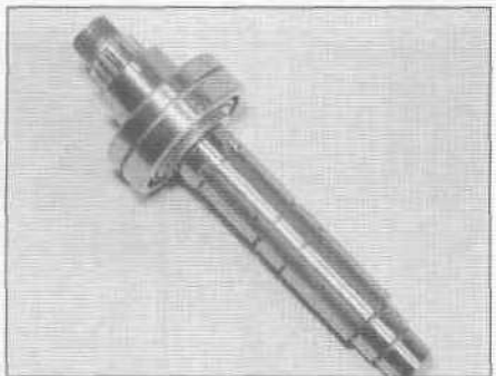
33.4p If the ball bearing is worn or damaged, have it replaced by a dealer service department or machine shop
