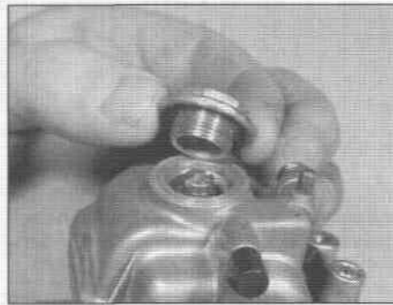
8.57 Remove the float chamber drain plug and its O-ring
