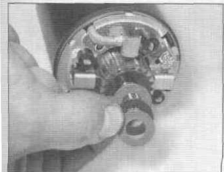
24.4a Take the shim(s) off each end of the starter...
