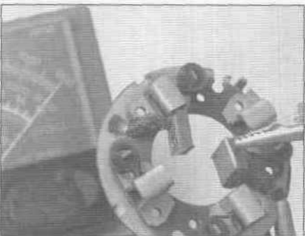
24.12 There should be almost no resistance (0 ohms) between the brushes and the brush plate
