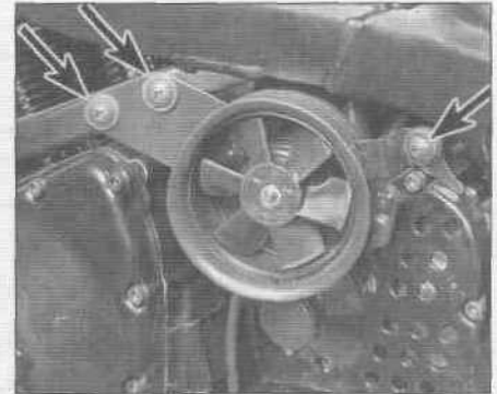
28.6 The fairing fan is secured by screws (arrowed) (Katana 600/GSX600F shown)
