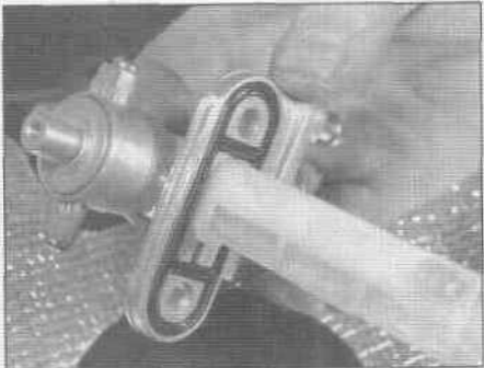
11.9b Replace the flange O-ring if it's brittle or deteriorated
