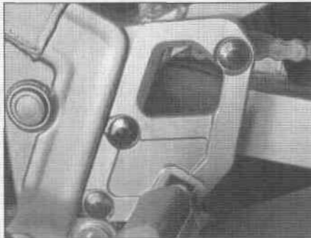
3.1b The footpeg brackets are bolted to the frame (Katana 1100/GSX1100F shown)
