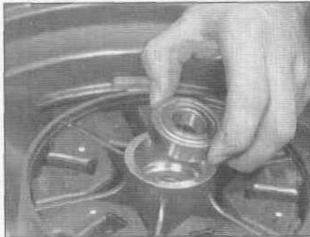
15.13b ... then install the remaining bearing
