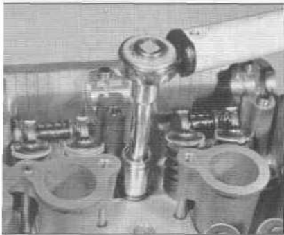
13.18c Tighten the head nuts in sequence to the correct torque
