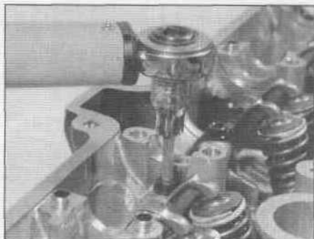
10.41 Tighten the rocker shaft lockbolts
