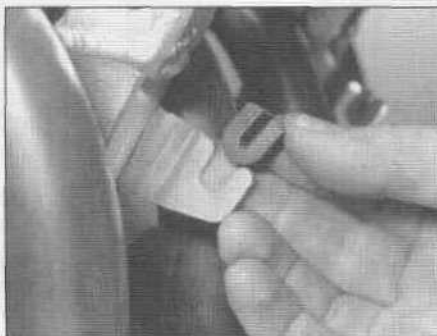
7.8 Replace the rubber vibration mounts if they're cracked, worn or compressed
