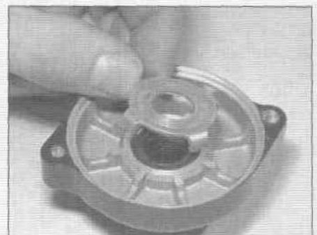
24.14 Lift the seal cover off to inspect the seal and needle roller bearing (if equipped)
