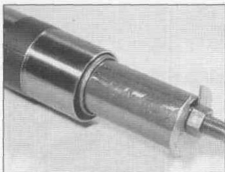
8.78b Use the Suzuki special tool or a washer with a slot cut in it to compress the spring
