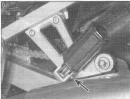
3.1a To detach a footpeg from the bracket, remove the C-clip and push out the pivot pin (arrowed) (Katana 1100/GSX1100F shown)
