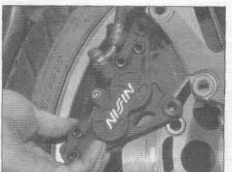
4.4b ... and lift the caliper off (late GSX-R1100 shown)
