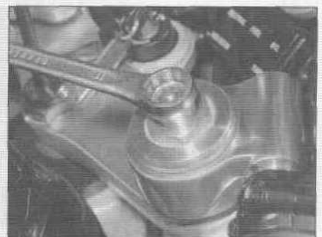
15.10a Turn the preload adjuster with a wrench to change spring preload
