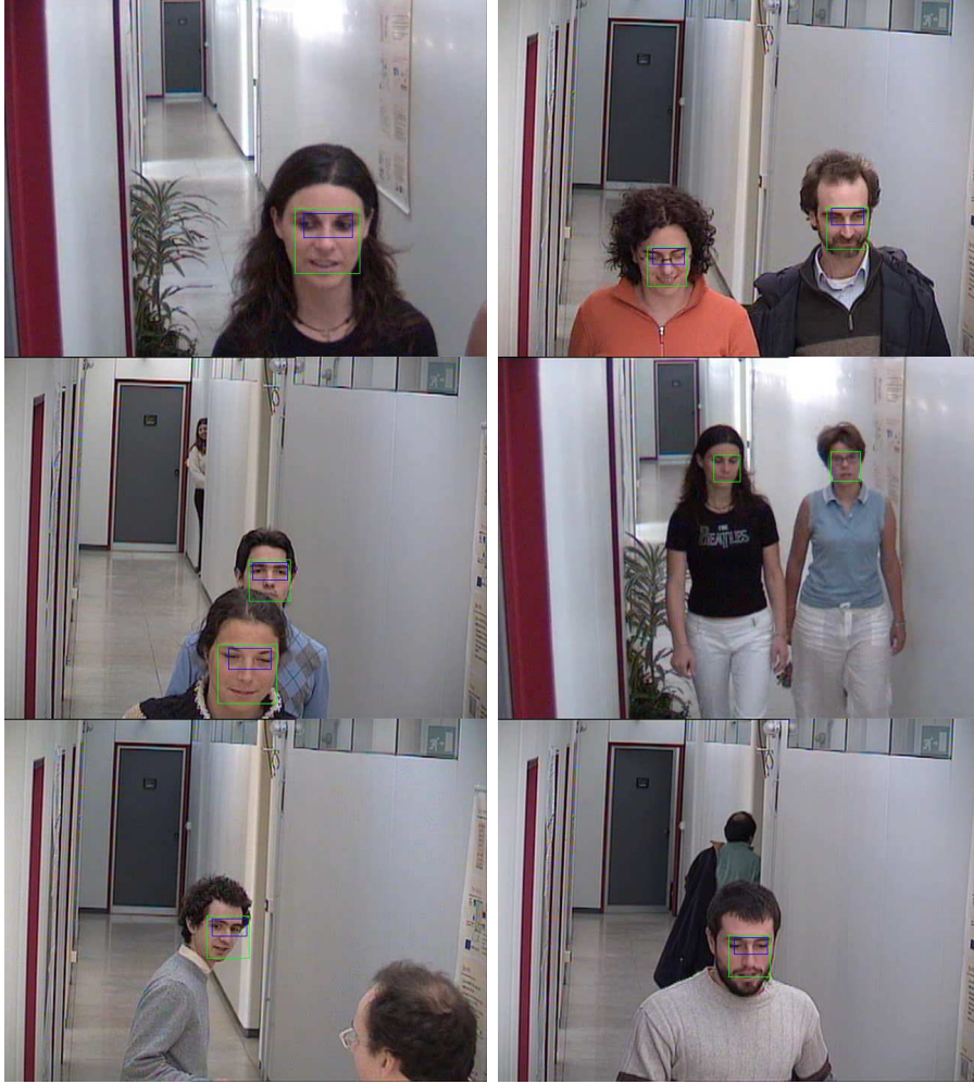
Fig. 19. Face and eye detection on sample frames acquired by our monitoring system: detected faces are marked in green, detected eye regions in blue. The minimum face size is of 19 \times 19 pixels, while the minimum eye region size is of 20 \times 40 pixels.
