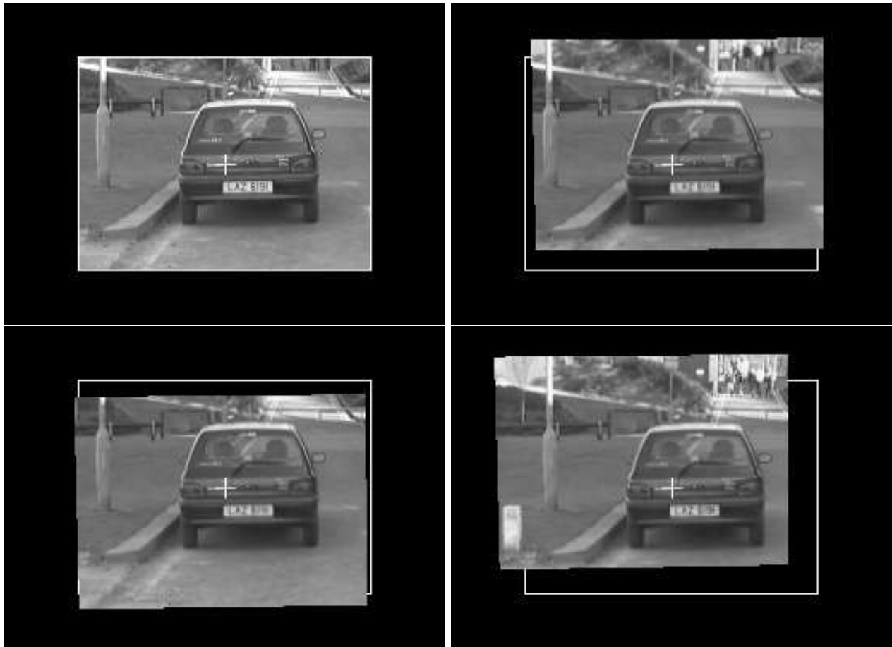
Figure 14: Frames (0, 35, 45, 89) stabilized from the sequence Clio. The first one is the reference frame.
