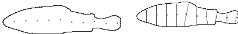
Figure 3: Illustration of length/width estimation: (a) initial skeleton points (column midpoints), (b) normal sections and final skeleton points.
