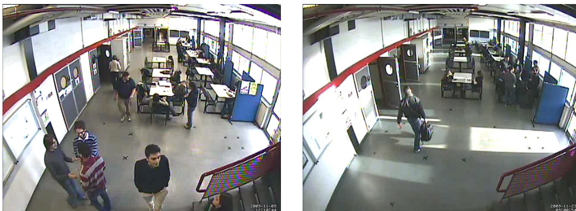
Figure 6.2: Sample frames acquired by the surveillance camera, showing the potentially complex conditions of the observed environment: the crowd level differs depending on the temporal interval considered, while the illumination is strongly affected by physical properties of the environment, in particular the presence of windows along the right wall.
