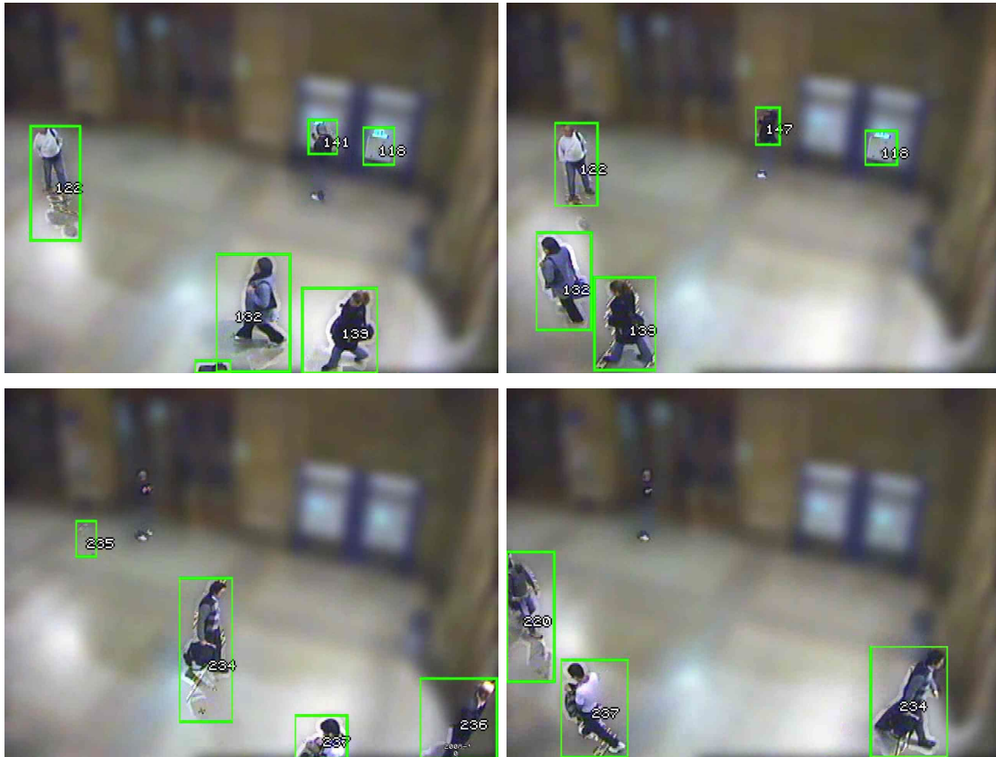
Figure 3.10: Sample frames of a real video-surveillance scenario (to keep the location secret, we only show the targets, smoothing the background). First and second images show multiple targets correctly maintained during time; in the others two people (identifiers 234 and 237) go towards each other, meeting and then splitting. The identities are re-associated.
