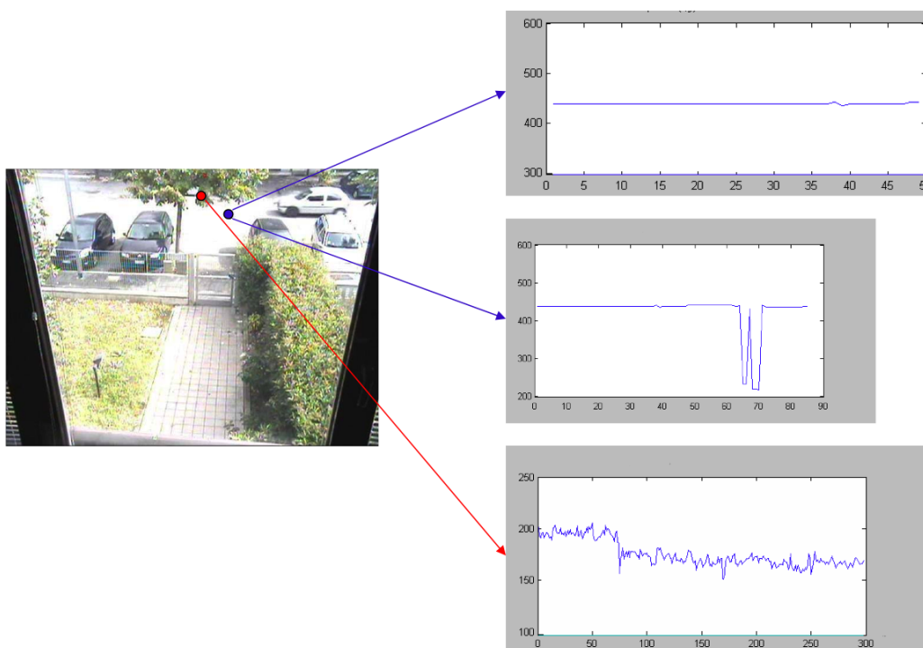
Figure 2.3: Pixels temporal evolutions with different characteristics: the blue arrow indicates a road pixel showing a rather stable value only temporarily affected by a significant variation due to car passage. An example of multiple background, instead, is provided by the red pixel, being an element of tree or road alternatively, due to the wind influence.
