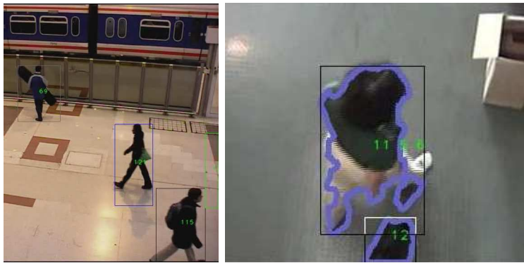
Figure 3: Examples of blob tracking: on the left multiple targets, on the right a static blob parts from a moving one.
