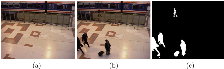
Figure 1: A reference frame (a) represents the background in the change detection method: the current scene (b) is subtracted from it to detect the moving foreground (c).
