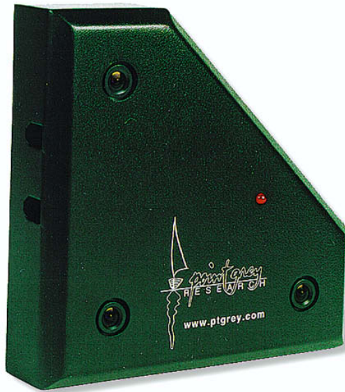
Figure 4: Digiclops color 3D camera, made by Point Grey Research and used by the Microsoft Research Easy Living group to provide stereo-vision positioning in a home environment. Image courtesy of Point Grey Research Inc.
