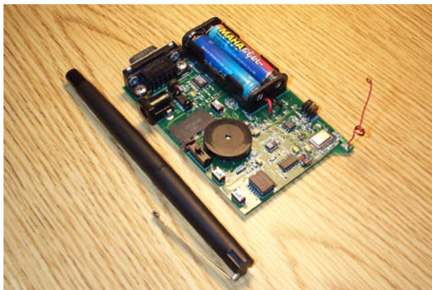
Figure 6: Prototype SpotON radio tag. These tags use radio signal attenuation to perform ad hoc lateration. Ad hoc clusters of tags cooperate to factor out measurement errors for all tag positions.
