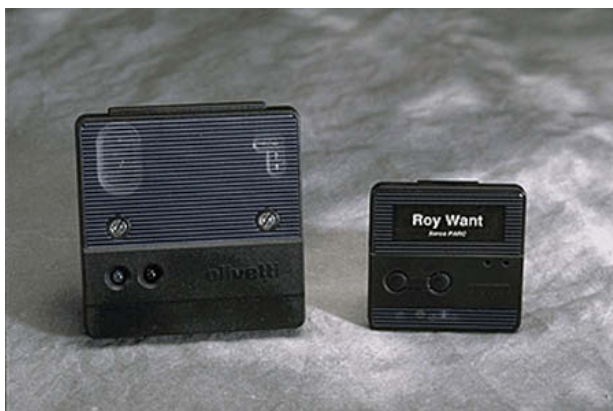
Figure 1: Olivetti Active Badge (right) and a base station (left) used in the system's infrastructure.
