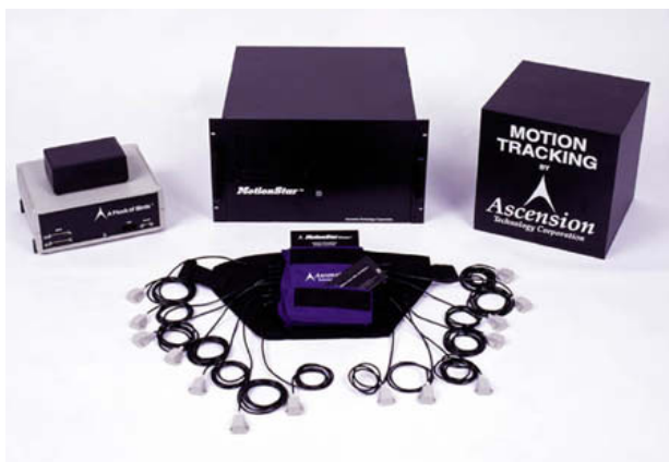
Figure 3: MotionStar DC magnetic tracker, a precision system used in motion capture for computer animation, tracks the position and orientation of up to 108 sensor points on an object or scene. Key components include (left and right) the magnetic pulse transmitting antennas and (center) the receiving antennas and controller. Image courtesy of Ascension Technology Corporation.
