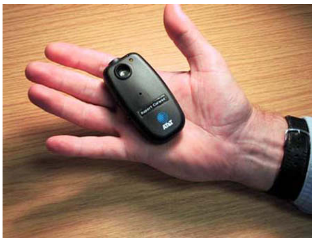
Figure 2: Mobile “Bat” of the At&T Cambridge Active Bat location system. Image courtesy of AT&T Laboratories Cambridge.
