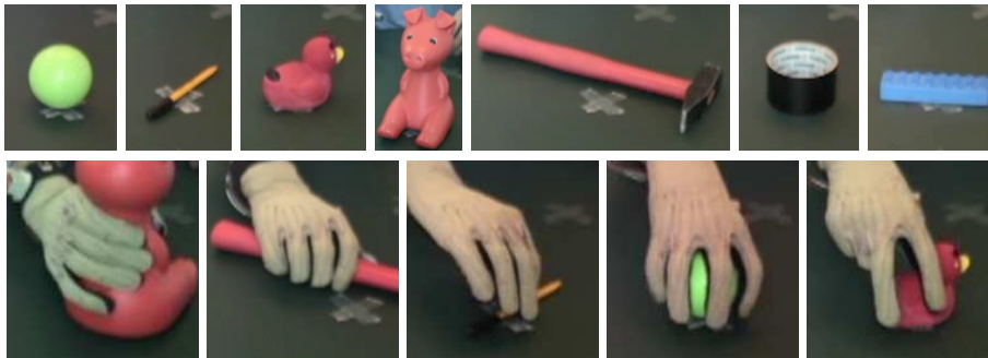
Figure 1: ( top row ) The 7 objects in the VMGdB. ( bottom row ) The 5 grasp types in the VMGdB (left to right: cylindric power grasp, flat, pinch grip, spherical and tripodal grip) applied to five of the considered objects.
