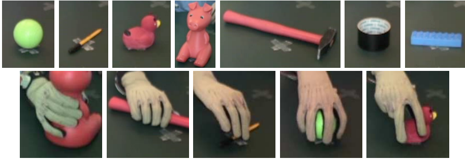
Fig. 2. Top row: the objects used in our experiments. Bottom, the grasp types we consider: (left to right) cylindrical power grasp, flat grasp, pinch grip, spherical and tripod grip.
