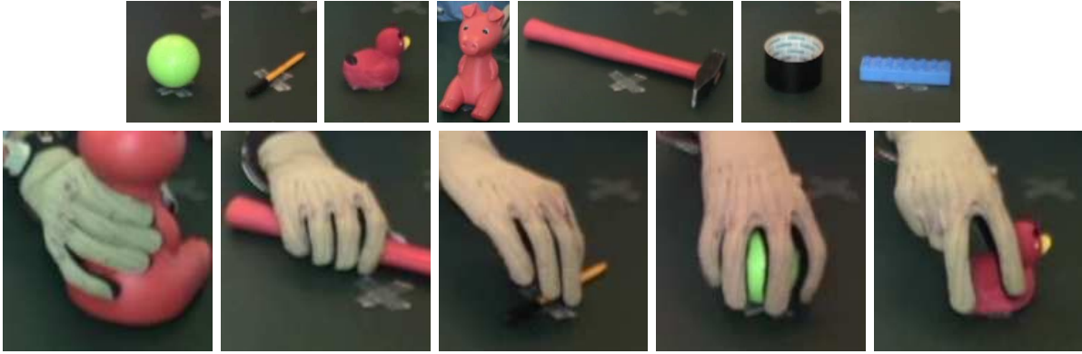
Figure 8.3: (Top row) The objects used in our experiments: (left to right) ball , pen , duck , pig , hammer , tape , lego . (Bottom row) The grasp types we consider: (left to right) cylindric power grasp , flat grasp , pinch grip , spherical and tripodal grip .
