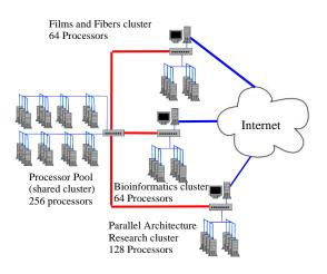
Figure 1: The Clemson Computational Mini-Grid
